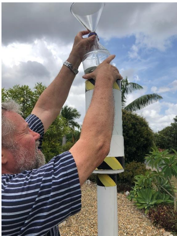
Figure 3: Removal of dust deposition gauge.
