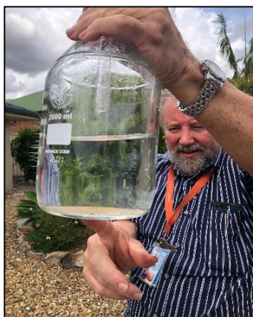
Figure 3: Dust gauge collection bottle contents.
