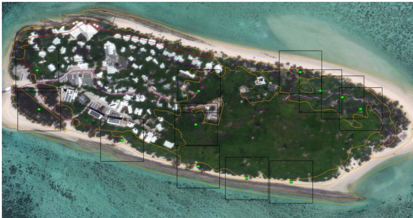
Figure 23: An example of existing site 1 data that fail due to the assessment area dimensions (criteria G or H). 1 the geo-referenced centre point for each site is represented by a green square and the surrounding box approx. 90m x 90m represents the area assessed by the model as representative of the site.
