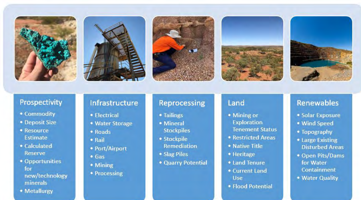
Figure 4: Overview of abandoned mine re-commercialisation and re-purposing criteria
