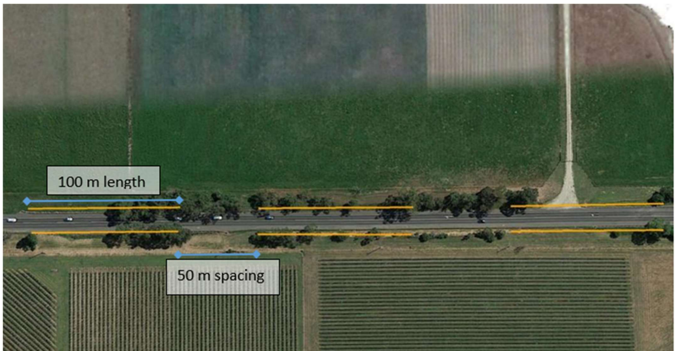
Figure 28. Example of how the six transects (orange lines) at a main road site are positioned, with a 50 m gap between them. Transects are laid out in pairs on opposite sides of the road (1 & 2, 3 & 4, 5 & 6).
