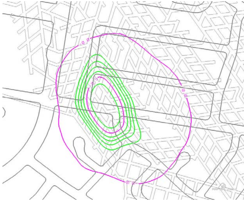
Figure A-75 Surface subsidence when pillars forced to fail with 66% roadway fill. Roadway void space is 3.0m with the model predicting 0.68m surface subsidence. Contour interval is 0.1m.
