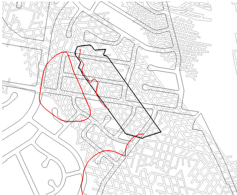
Figure A-76 Location of numerical model #2 together with surface subsidence contours from 1988 and 2008 events and seam level eastern boundary of failure predicted from 3D seismic.
