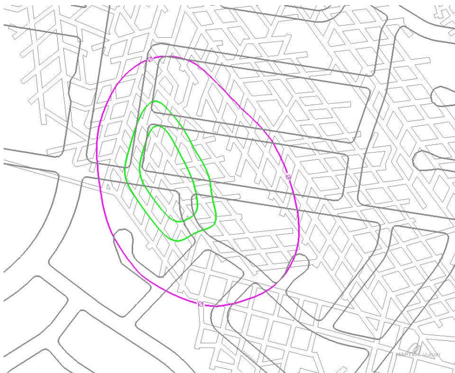
Figure A-70 Surface subsidence predicted by numerical model when pillars forced to fail with 83% roadway fill. Contour interval is 0.1m with maximum subsidence predicted as 0.22m.
