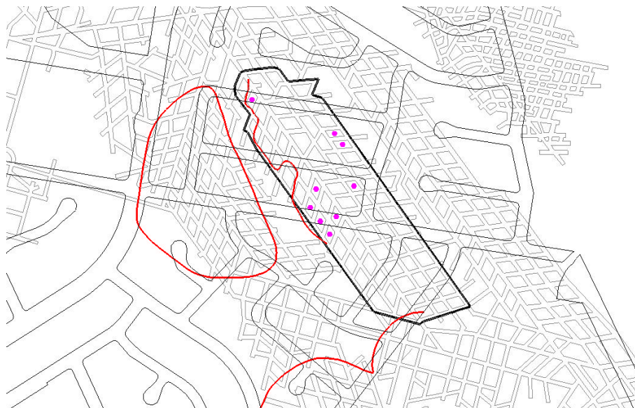
Figure A-79 Pillars predicted to have failed from Numerical model #2 with surface subsidence contours and inferred eastern limit of failed zone at seam level.
