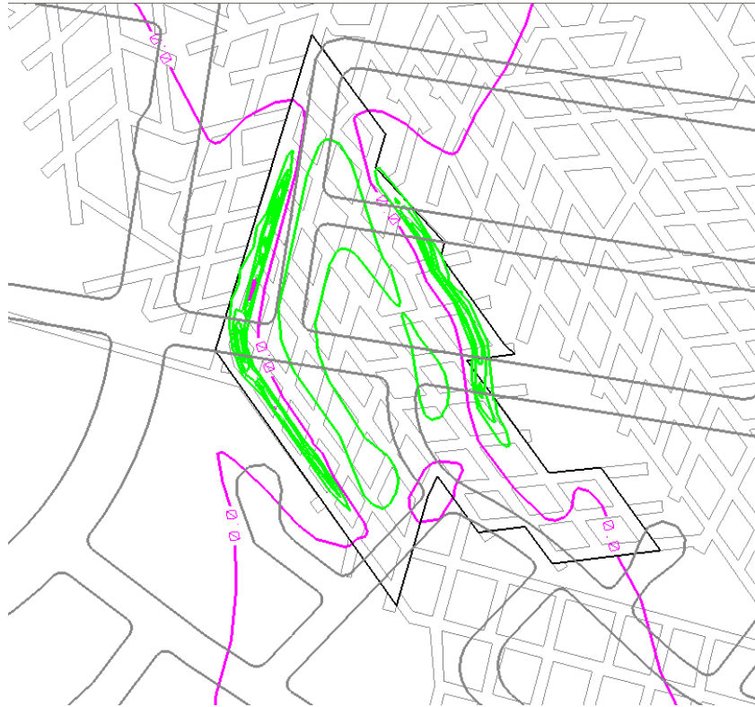
Figure A-71 Surface strain in east-west direction when pillars forced to fail resulting 0.22m surface subsidence. Maximum strain is 5mm/m and contour interval is 1mm/m.
