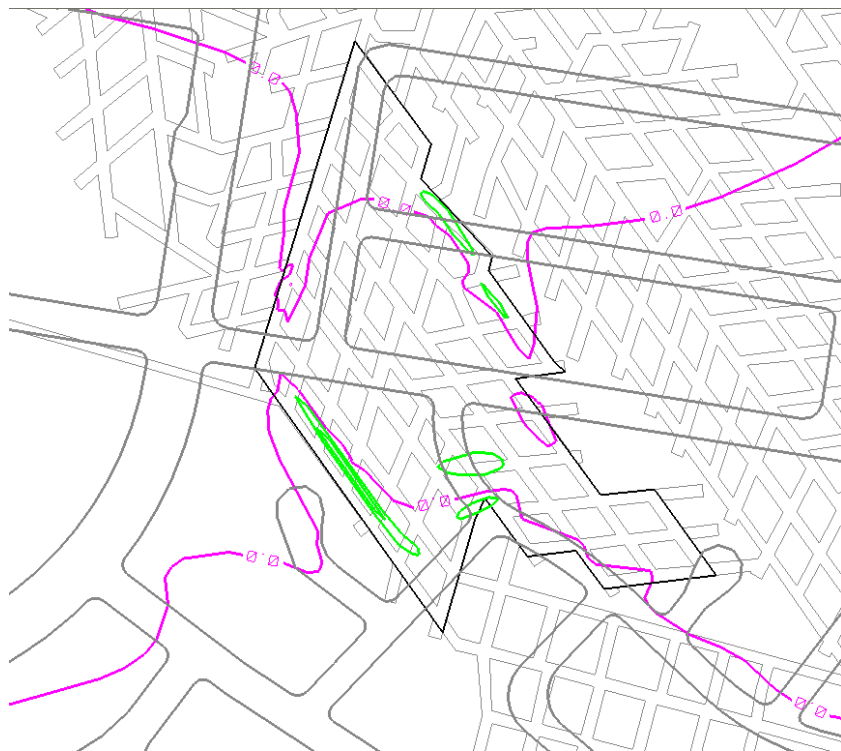
Figure A-72 Surface strain in north-south direction when pillars forced to fail resulting 0.22m surface subsidence. Maximum strain is 3mm/m and contour interval is 1mm/m.
