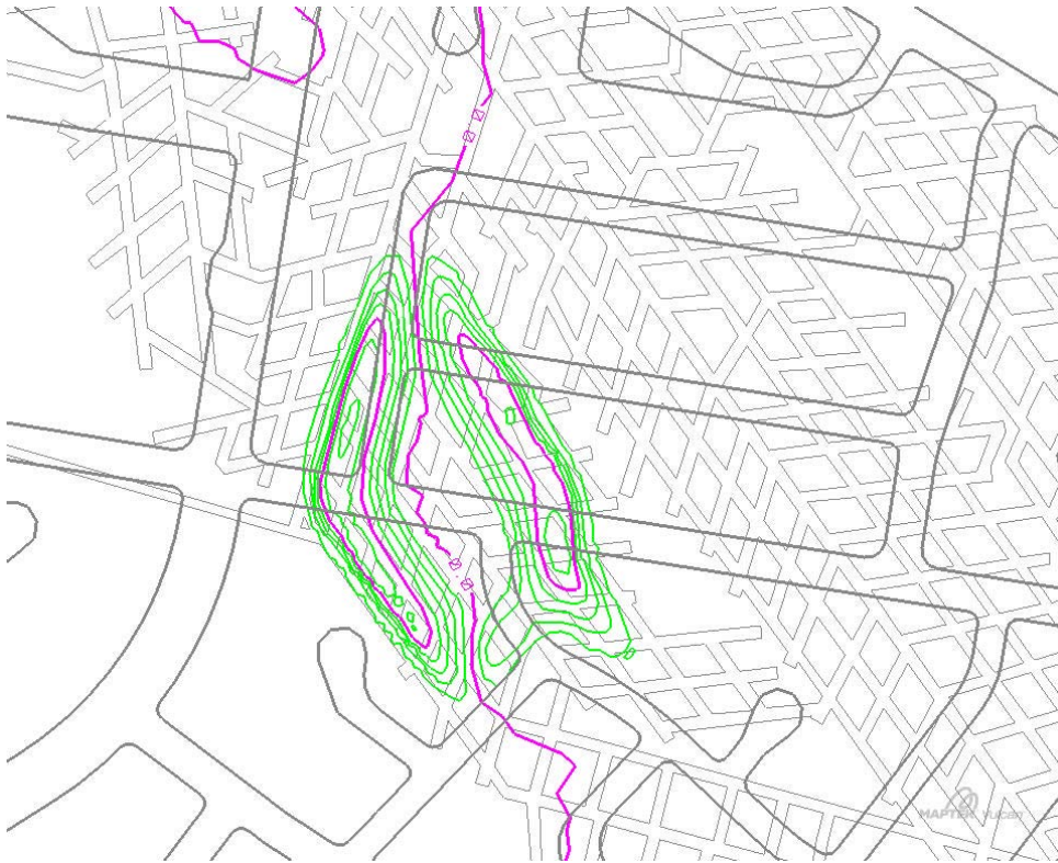
Figure A-73 Tilt in east-west direction. Units are mm/m and intervals are 1mm/m, maximum tilt is 7mm/m.
