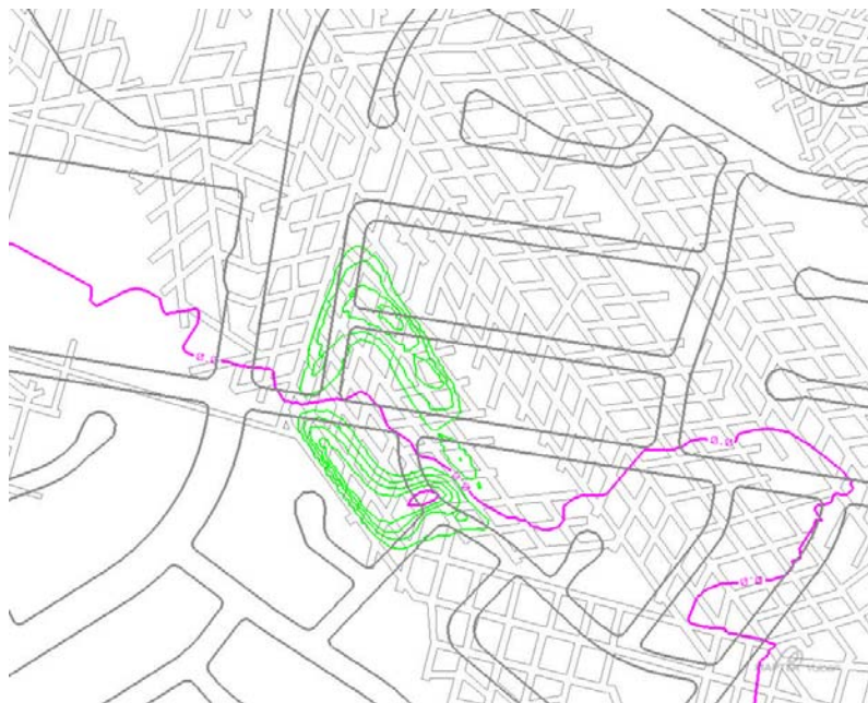
Figure A-74 Tilt in north-south direction. Units are mm/m and intervals are 1mm/m, maximum tilt is 5mm/m.
