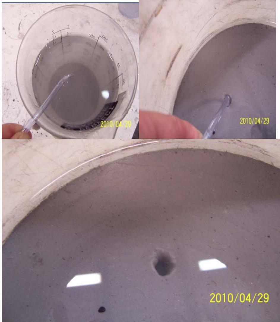
Figure B-30 Suction test by siphoning water from a submerged fly ash sediment
