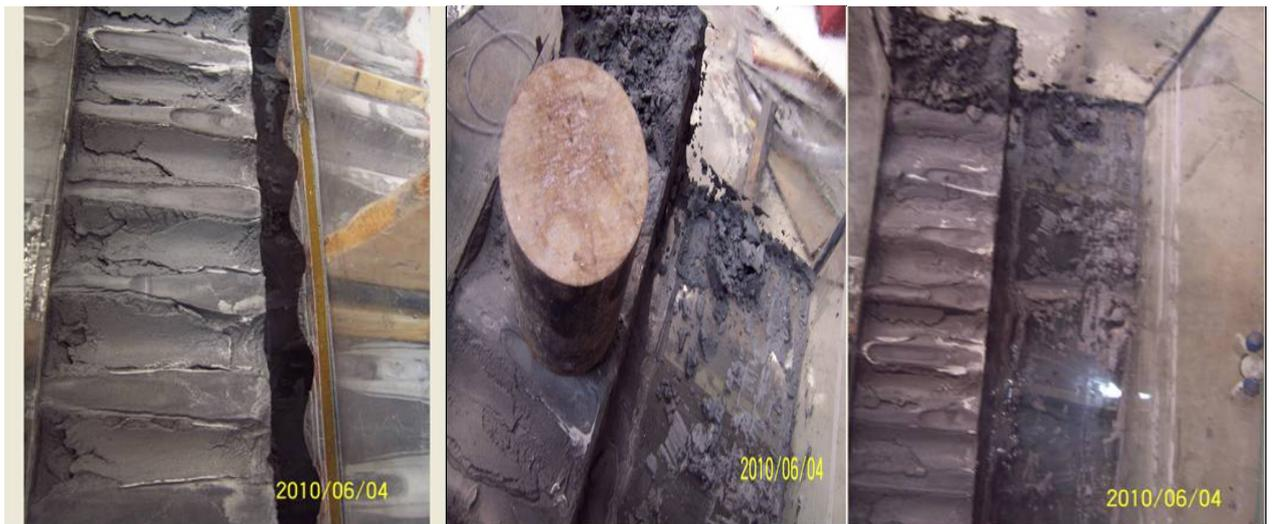
Figure B-58 Backfilling test of roadways with corrugated roofs – Under dry conditions still stable walls can remain even after formwork removal. A surcharge load has been added to check the wall vertical stability (middle photo)
