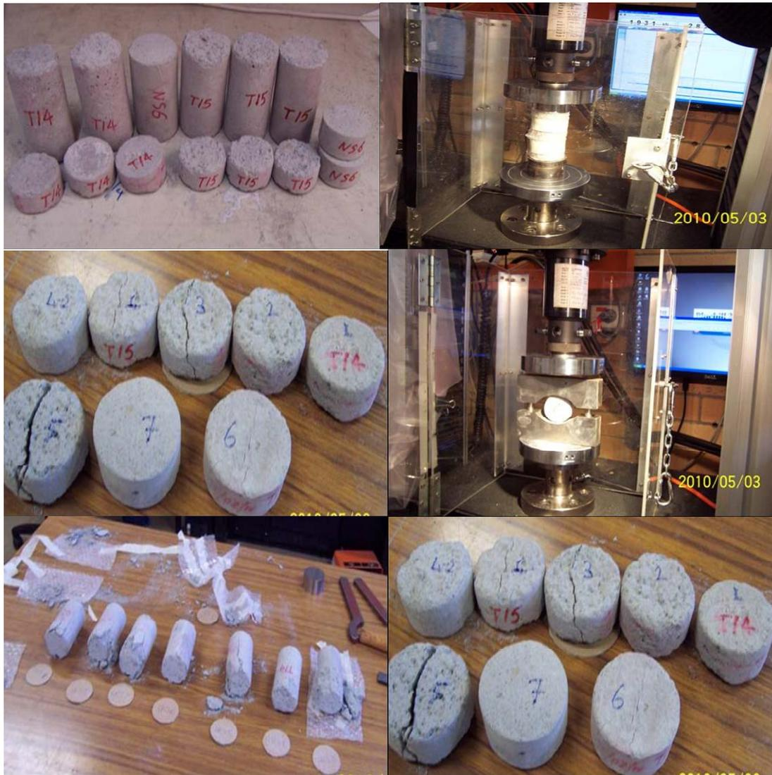
Figure B-60 Samples of cohesive fly ash used in compressive UCS and tensile BTS strength tests
