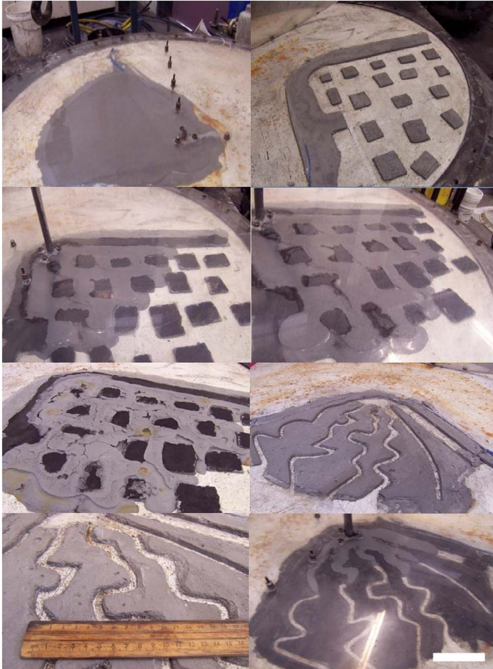
Figure B-39 Fly ash grout infill in a 4mm disc gap void (top left) and through wide voids and obstacles (top right and middle rows) and narrow curly paths (bottom row)
