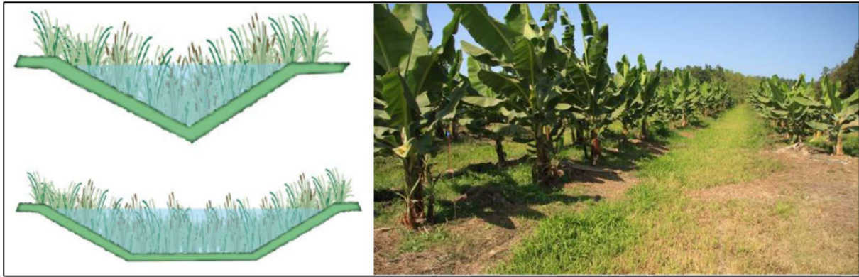
Figure 6: Left: Diagram to show cross sections of vegetated drains (top) and vegetated swales (bottom). Right: Example of a wide, vegetated spoon swale on a banana property (Source: Queensland Department of Environment and Science, WetlandInfo 2018b).
