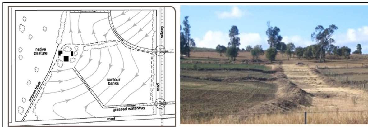
Figure 11: Left: Example of a contour bank layout on a banana farm (Source: figure 7.1, Chapter 7 Soil Conservation Guidelines). Right: Example of well-maintained contour banks on a Queensland farm (Source: Preventing and managing erosion ).
