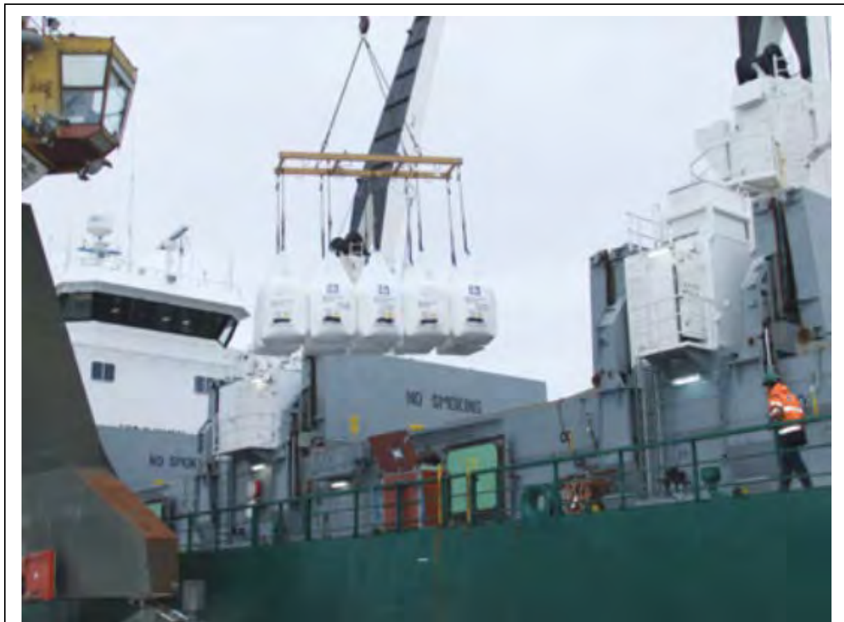
Photo 7-4 Typical lifting frame for loading bags.
