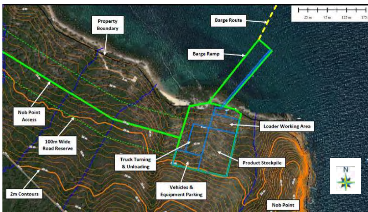
Figure 7-15 Nob Point barge ramp concept.
