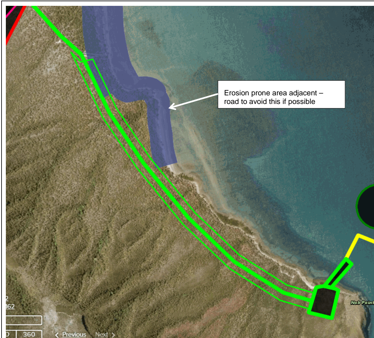
Figure 8-34 Erosion prone area adjacent to the Nob Point Transport Corridor.
