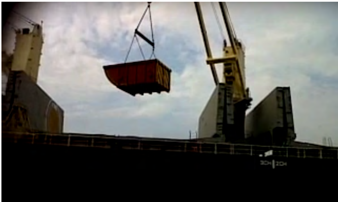
Photo 7-3 Typical steel skips being loaded by crane.
