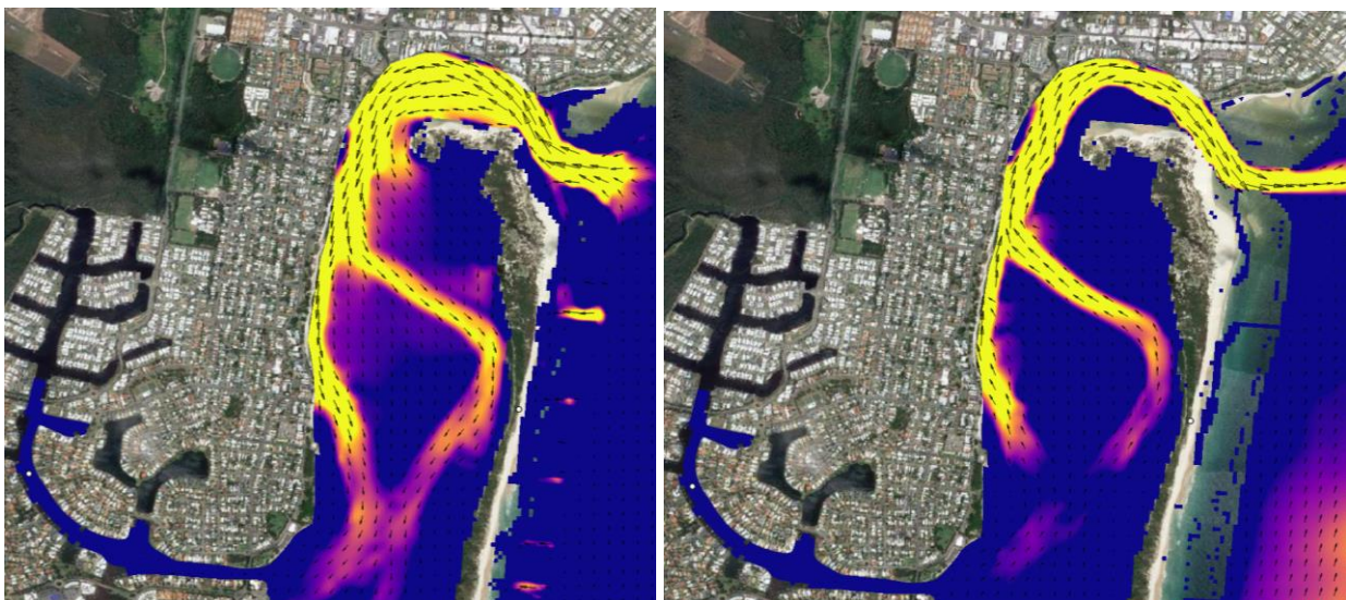
Figure 3.8 Peak flood tide (left) and ebb tide (right) for Pumicestone Passage for normal tide-only conditions.
