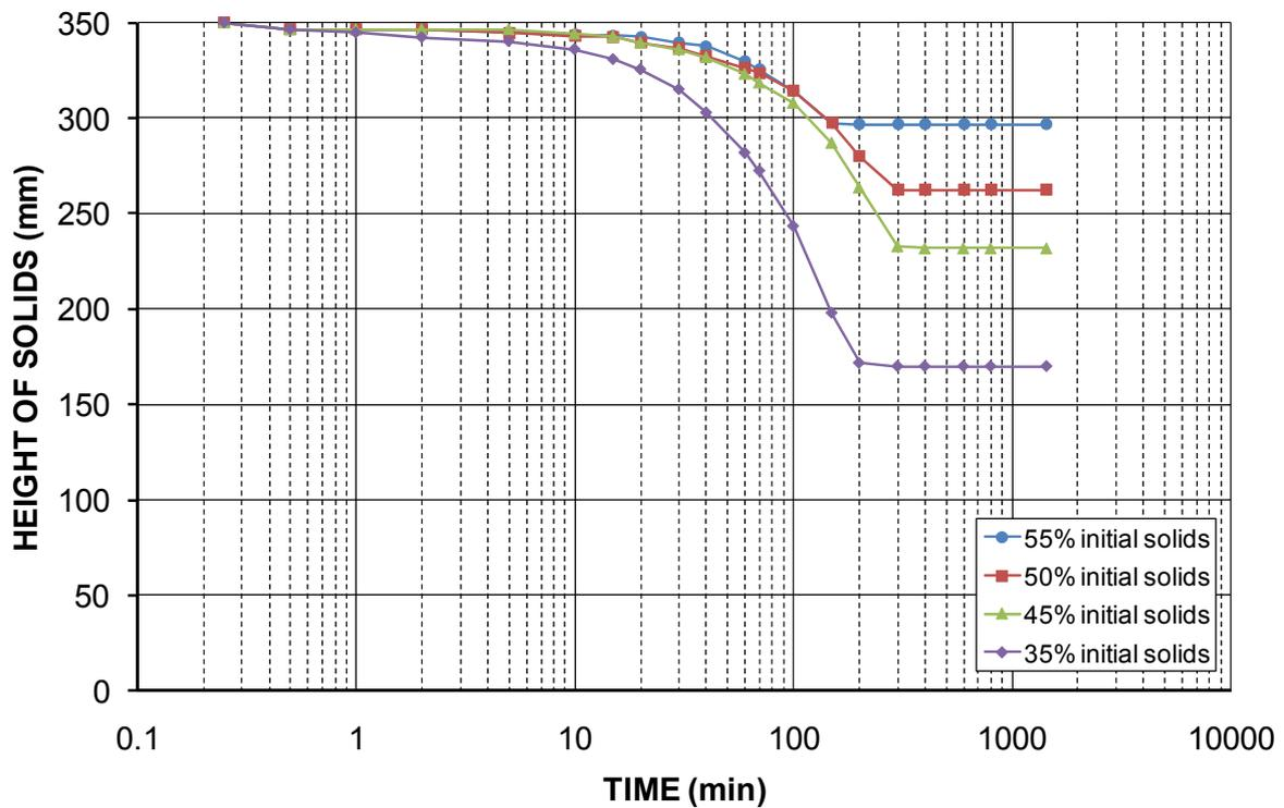
Figure 10 Settlement of Swanbank fly ash solids vs. Log<sub>10</sub> (Time) for various initial % solids
