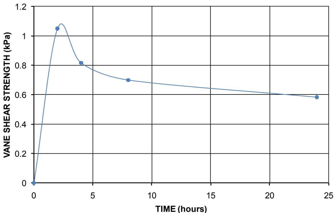
**Figure 17** Undrained vane shear strength of settling Swanbank fly ash solids vs. Time
