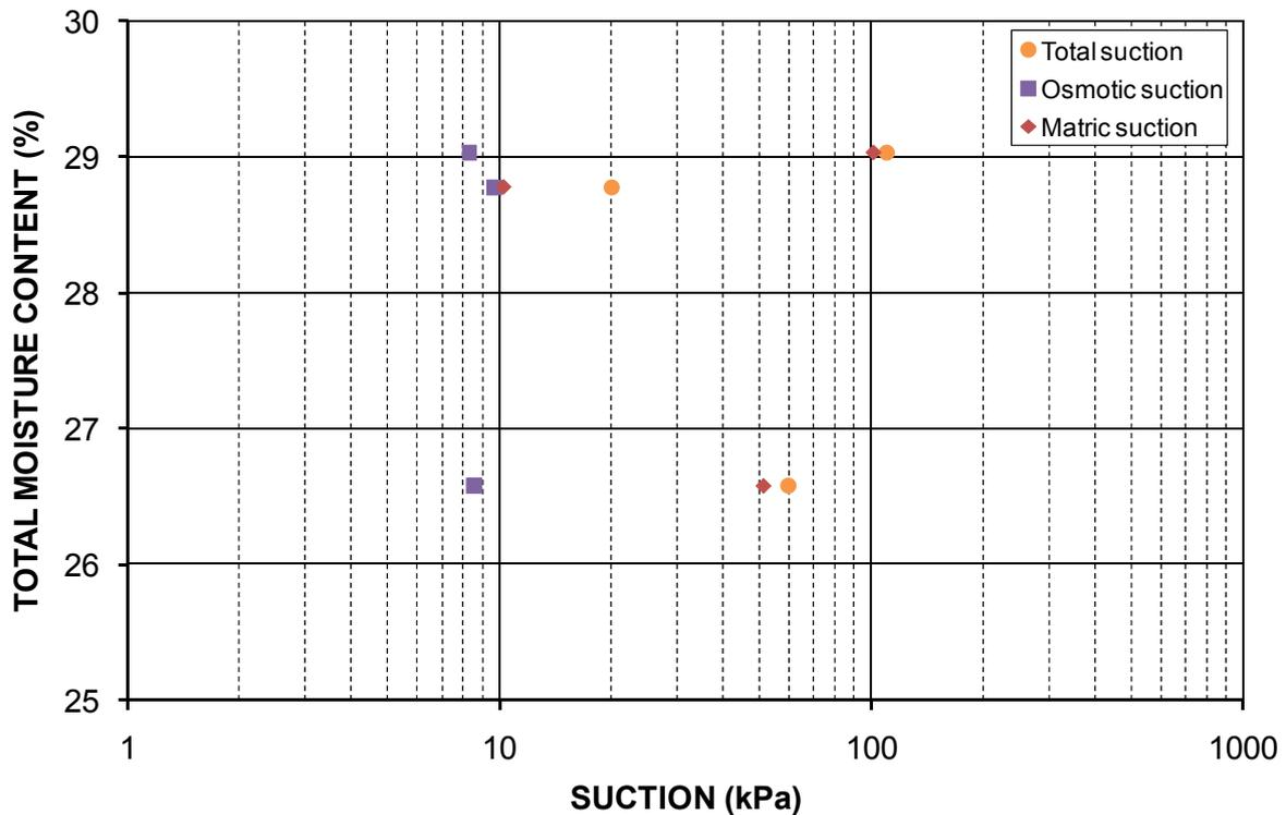
Figure 8 Total moisture content vs. Suction for Swanbank fly ash drum samples
