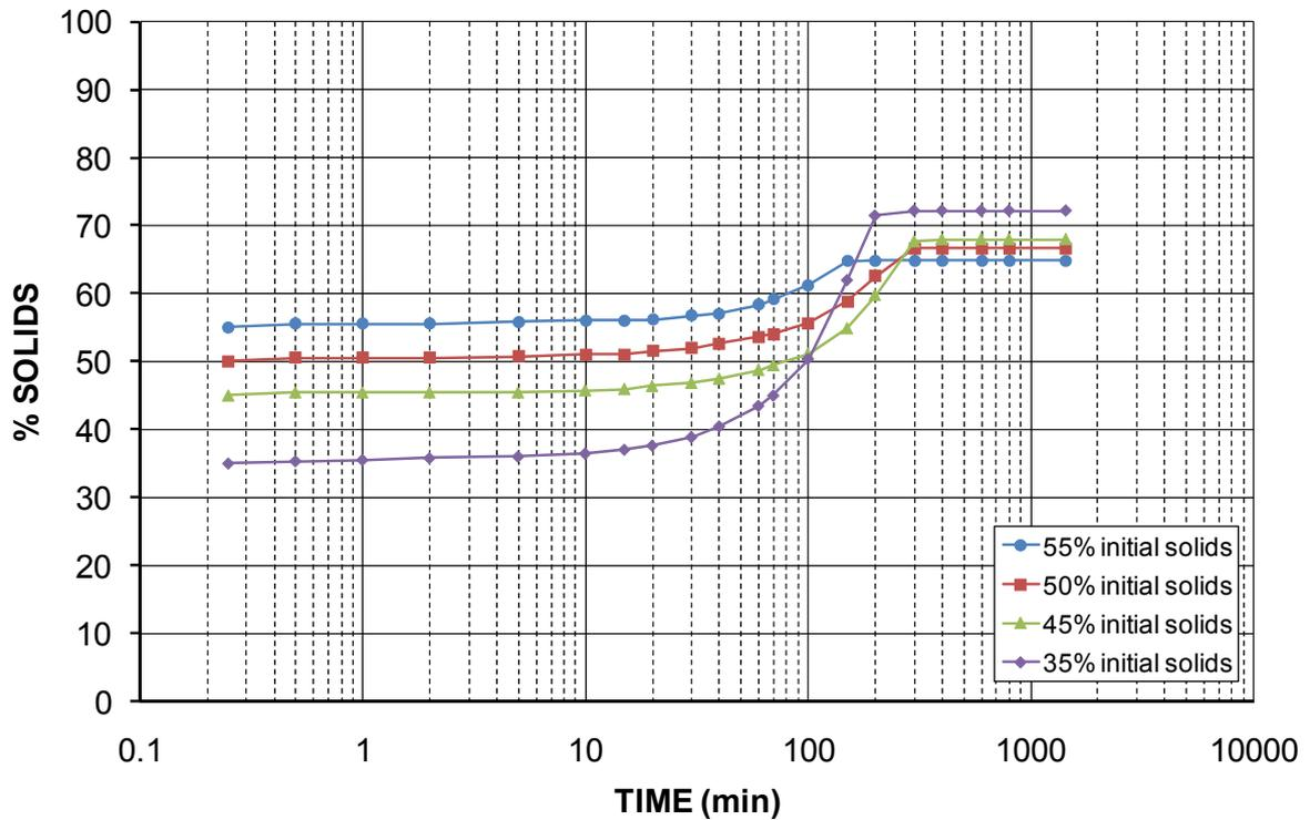
Figure 12 Average % Solids of settling Swanbank fly ash solids vs. Log<sub>10</sub> (Time) for various initial % solids
