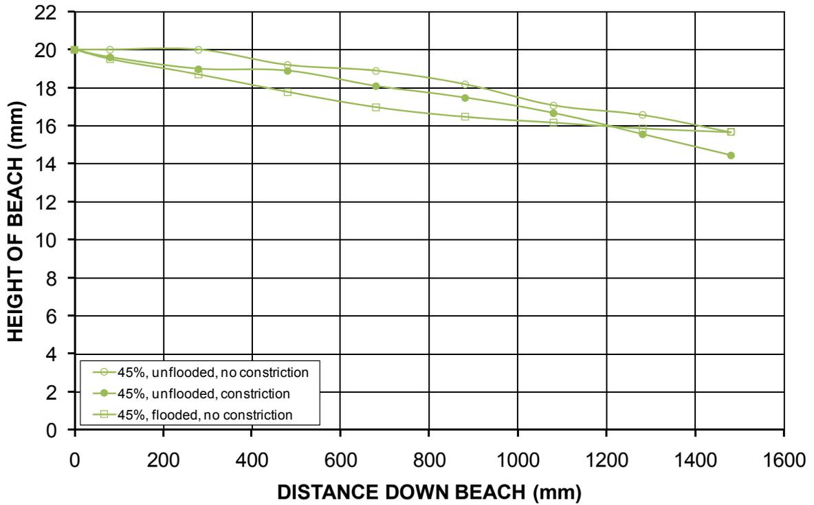
**Figure 30** Summary of open-ended laboratory flume beach profiles for Swanbank fly ash
