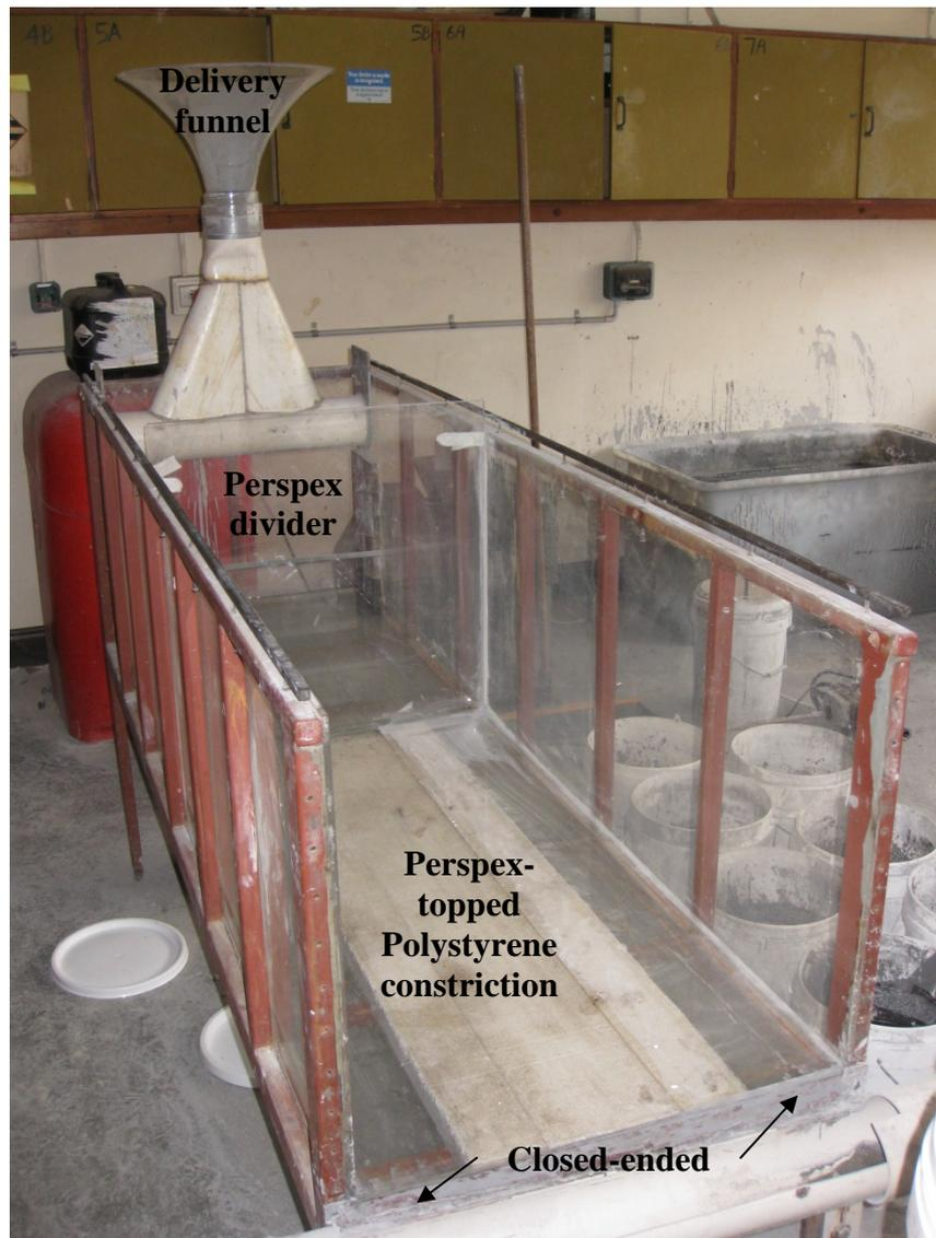
**Figure 5** Laboratory flume showing central constriction topped with Perspex, and Perspex divider
