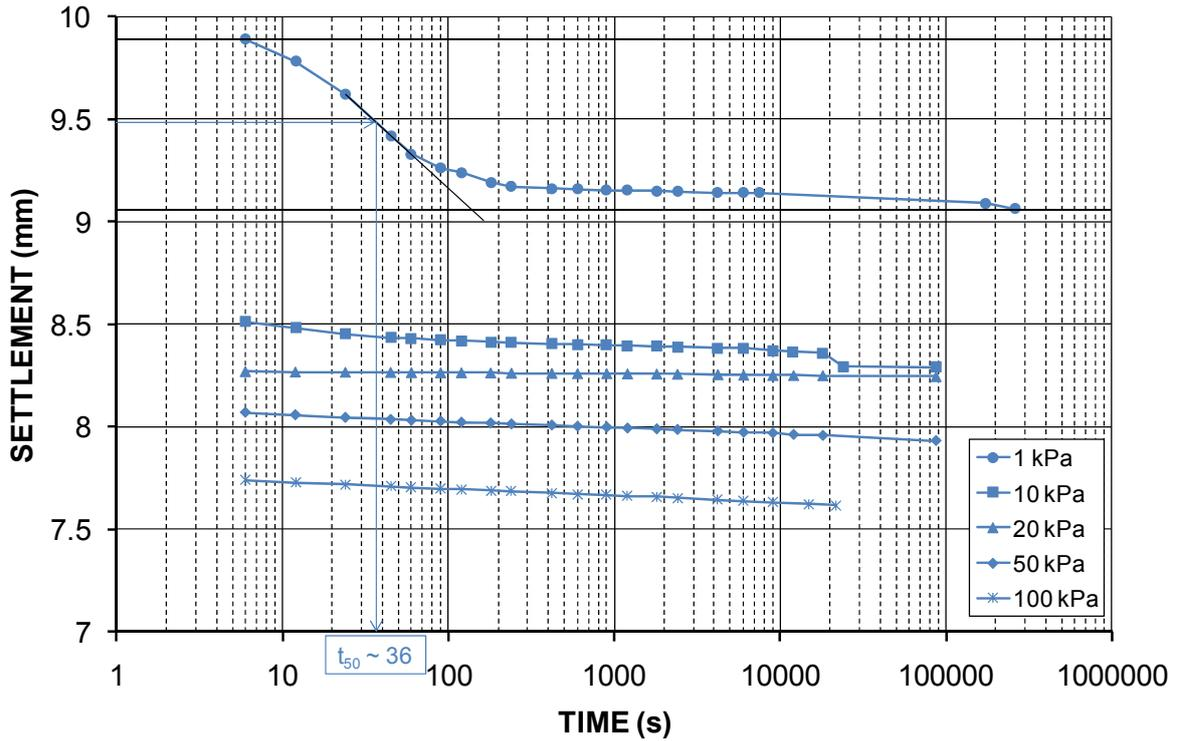
Figure 21 Oedometer settlement vs.  $\text{Log}_{10}$  (Time) for settled Swanbank fly ash at various effective stresses
