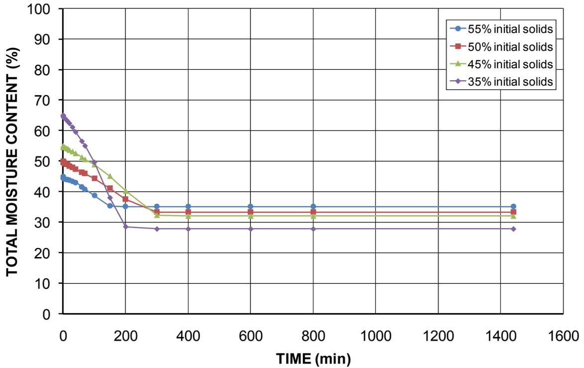
Figure 13 Average total moisture content of settling Swanbank fly ash solids vs. Time for various initial % solids
