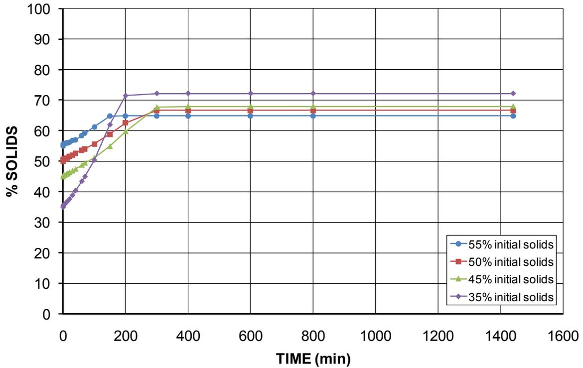
Figure 11 Average % Solids of settling Swanbank fly ash solids vs. Time for various initial % solids
