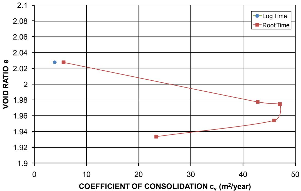
**Figure 23** Void ratio vs. Coefficient of Consolidation for Swanbank fly ash
