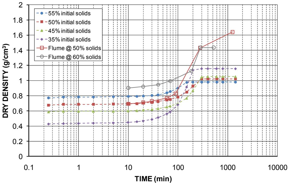
**Figure 39** Comparison of Swanbank fly ash average dry density on settling column, and flume testing under water and under a high head
