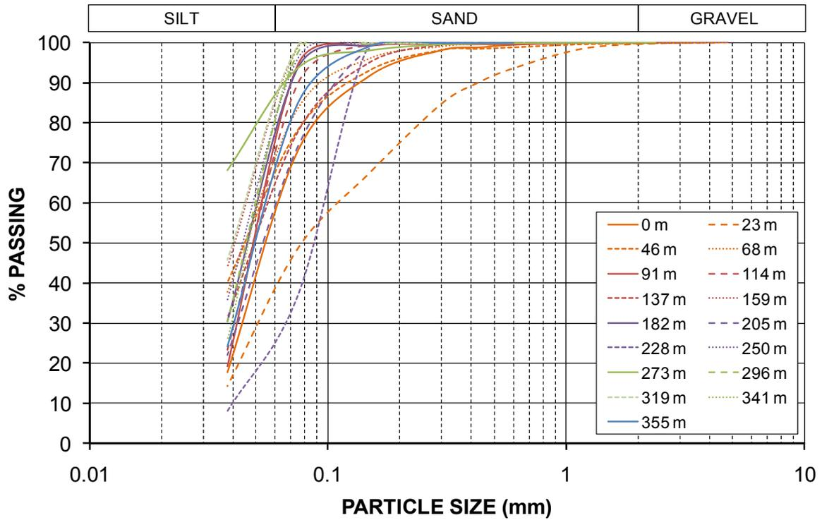
**Figure 42** Particle size distribution curves down field beach profile for sub-aerial, unconstricted deposition of Swanbank fly ash
