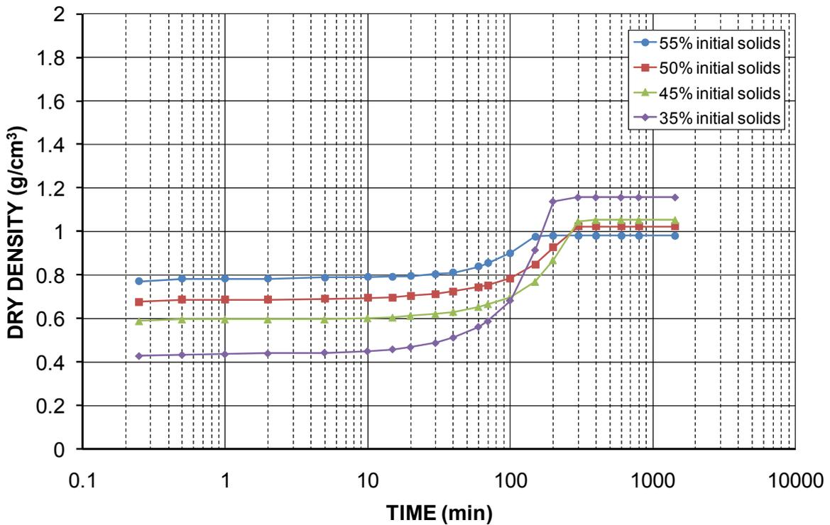
Figure 16 Average dry density of settling Swanbank fly ash solids vs.  $\text{Log}_{10}$  (Time) for various initial % solids
