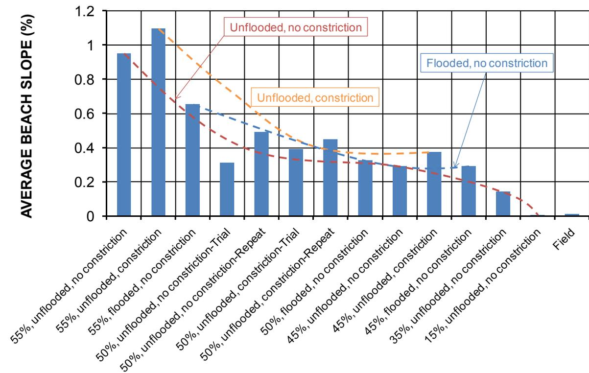
**Figure 46** Comparison of average beach slopes of laboratory and field beach profiles for Swanbank fly ash
