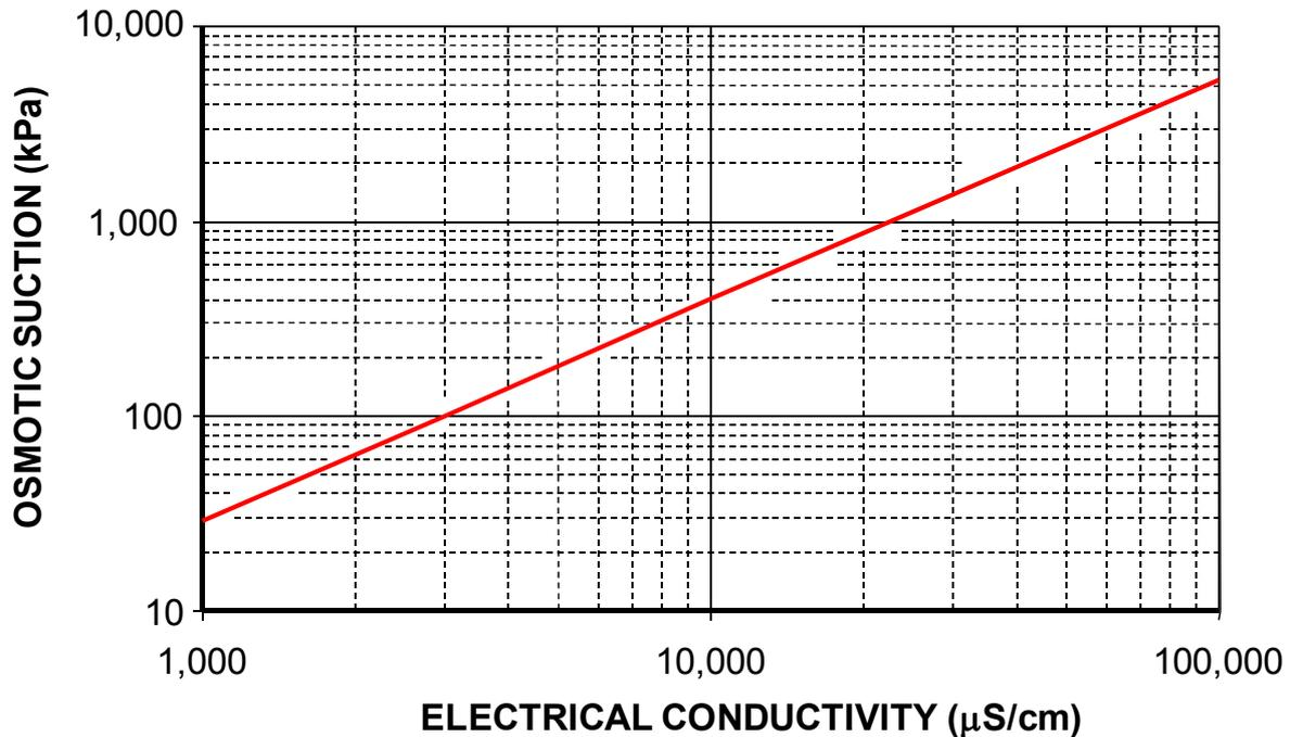
**Figure 4** Correlation between osmotic suction and Electrical Conductivity (at 25oC; after USDA, 1954)<sup>6</sup>
