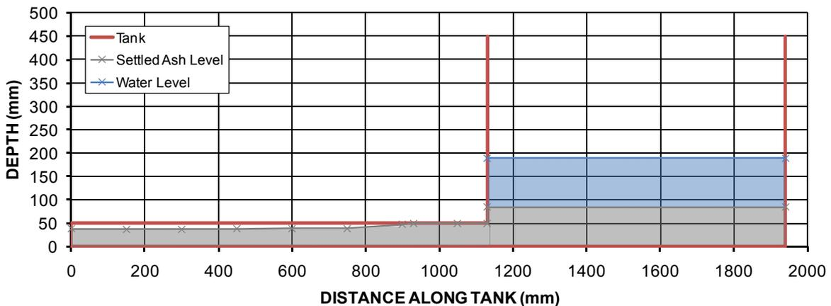
**Figure 34** Constricted backfilling, under water and a low head of Swanbank fly ash slurry, initially at 50% solids
