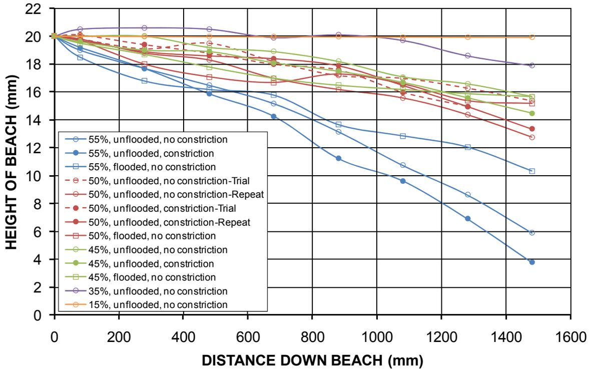
**Figure 27** Summary of open-ended laboratory flume beach profiles for Swanbank fly ash
