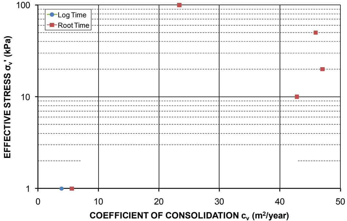
**Figure 24** Effective stress vs. Coefficient of Consolidation for settled Swanbank fly ash
