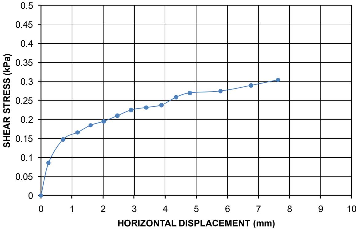
**Figure 18** Direct shear box shear strength of settled Swanbank fly ash solids vs. Horizontal displacement
