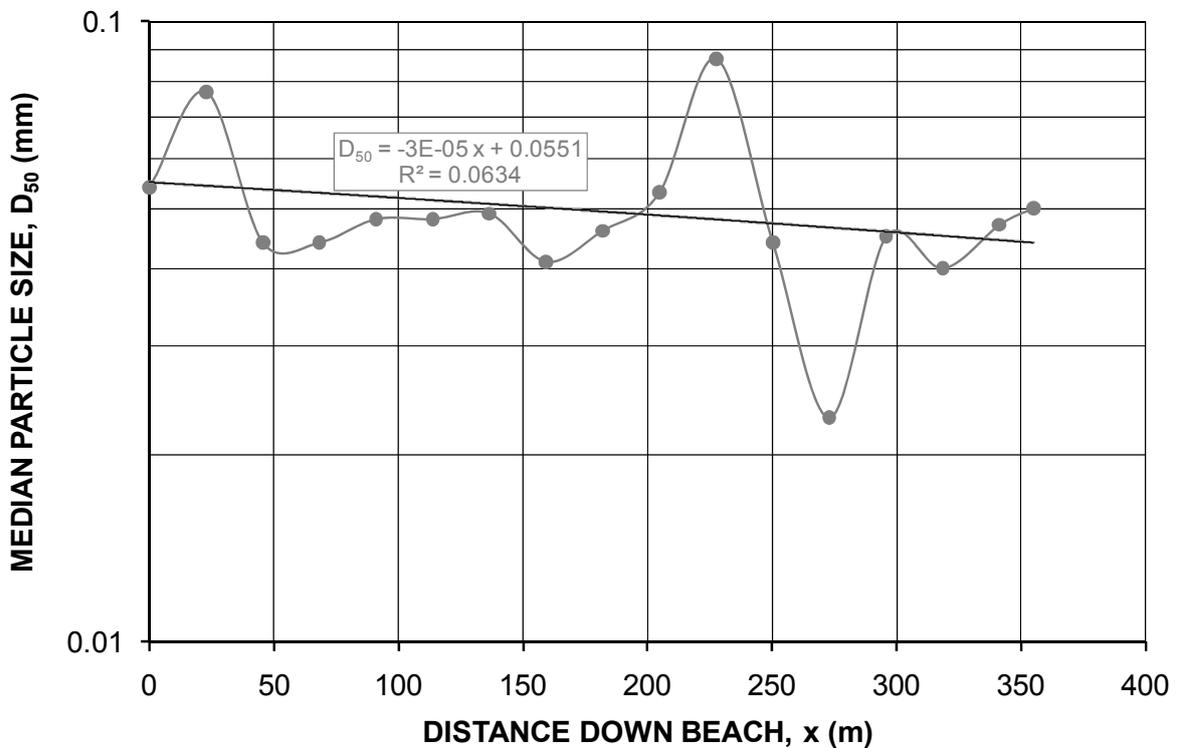
**Figure 43** Median particle size down field beach profile for sub-aerial, unconstricted deposition of Swanbank fly ash
