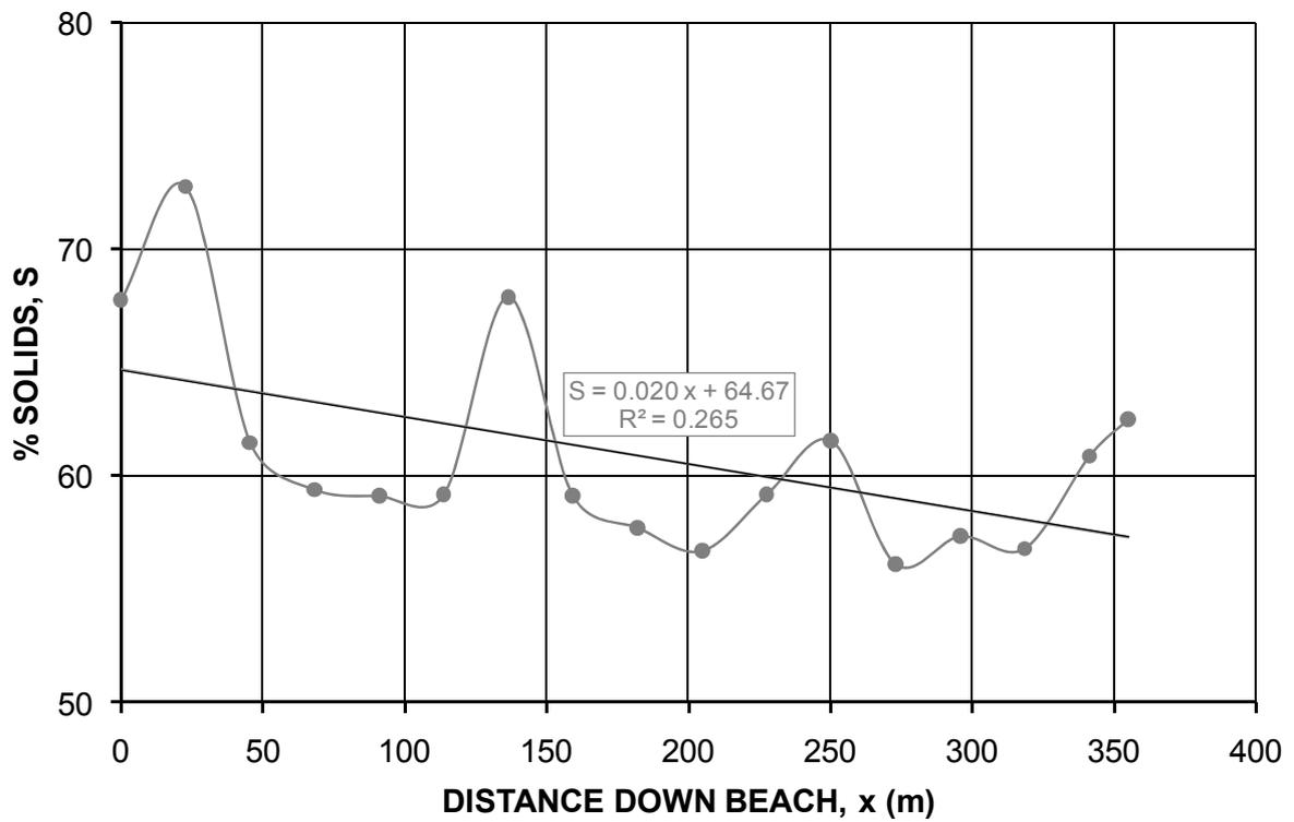
**Figure 45** % Solids down field beach profile for sub-aerial, unconstricted deposition of Swanbank fly ash
