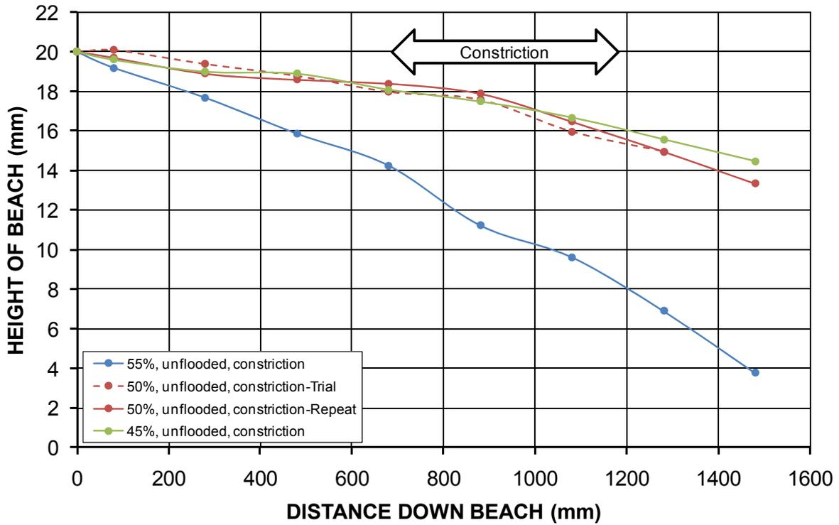
**Figure 32** Laboratory flume test beach profiles for unflooded, constricted deposition of Swanbank fly ash
