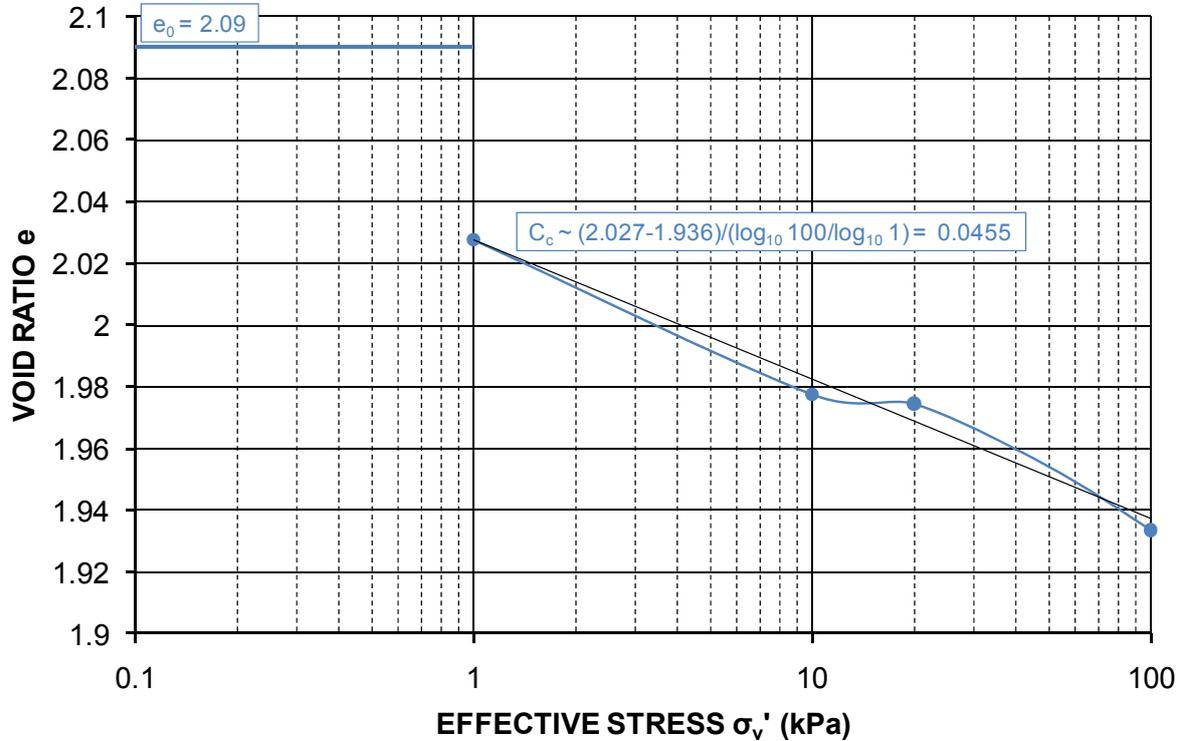
**Figure 20** Oedometer plot of Void ratio vs. Effective stress for settled Swanbank fly ash
