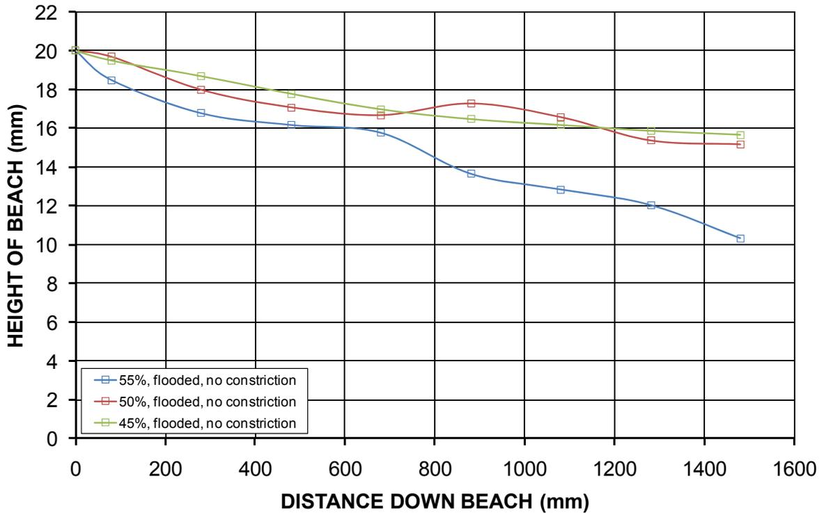
**Figure 33** Laboratory flume test beach profiles for flooded, unconstricted deposition of Swanbank fly ash
