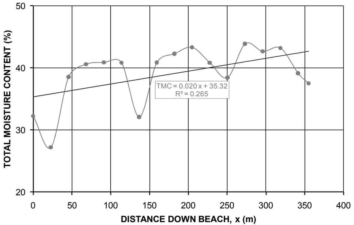
**Figure 44** Total moisture content down field beach profile for sub-aerial, unconstricted deposition of Swanbank fly ash
