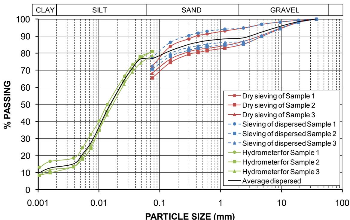
**Figure 7** Particle size distribution curves for Swanbank fly ash
