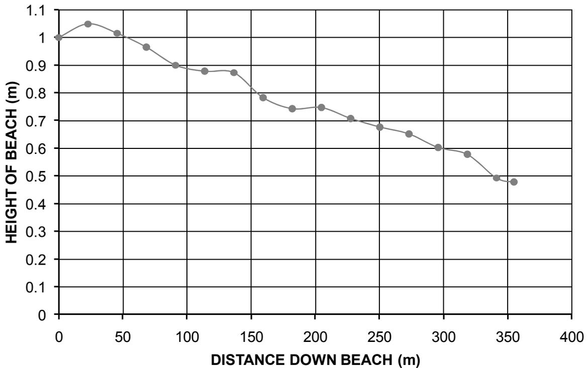
**Figure 40** Field beach profile for sub-aerial, unconstricted deposition of Swanbank fly ash
