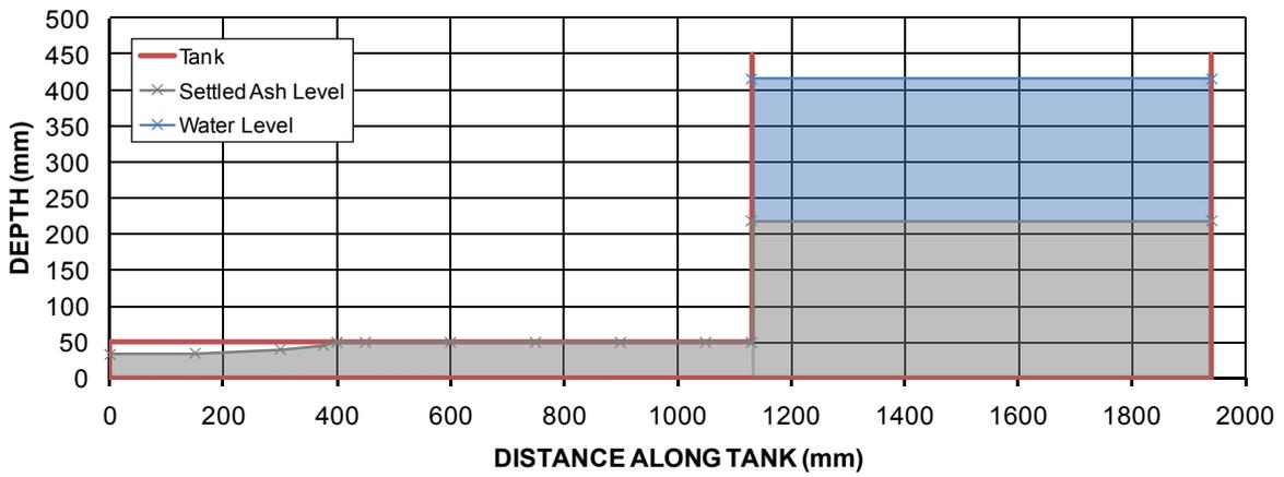
**Figure 35** Constricted backfilling, under water and a high head of Swanbank fly ash slurry, initially at 50% solids
