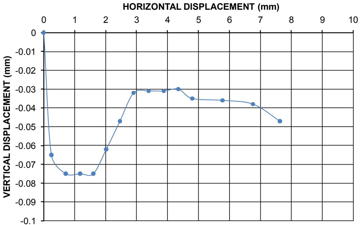
**Figure 19** Direct shear box vertical displacement (settlement) of settled Swanbank fly ash solids vs. Horizontal displacement
