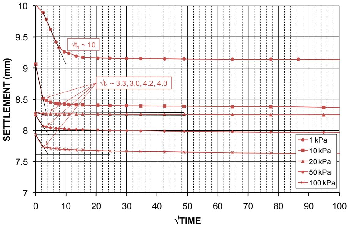
Figure 22 Oedometer settlement vs.  $\sqrt{\text{Time}}$  for settled Swanbank fly ash at various effective stresses
