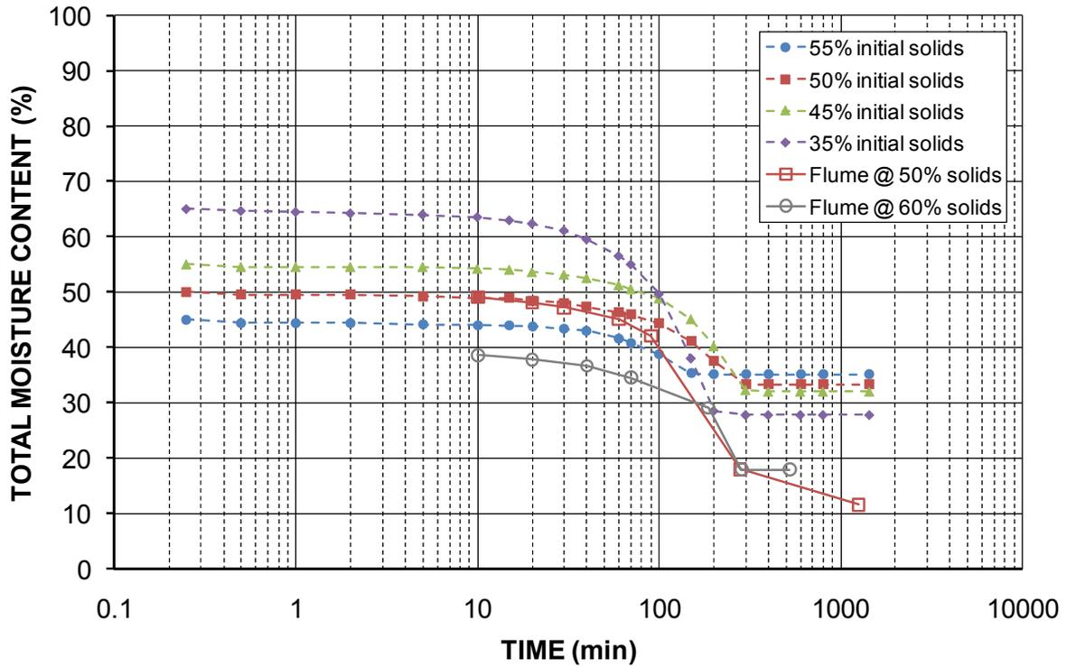
**Figure 38** Comparison of Swanbank fly ash average total moisture contents on settling column, and flume testing under water and under a high head
