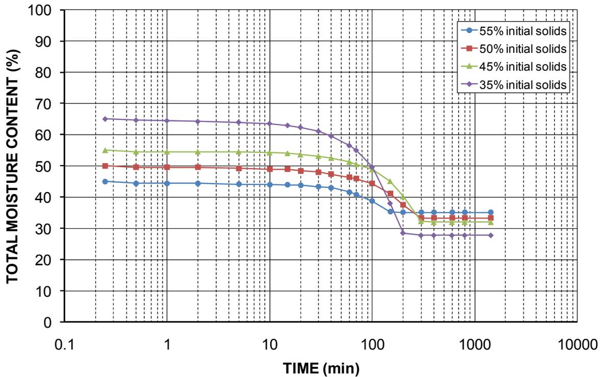
Figure 14 Average total moisture content of settling Swanbank fly ash solids vs. Log<sub>10</sub> (Time) for various initial % solids
