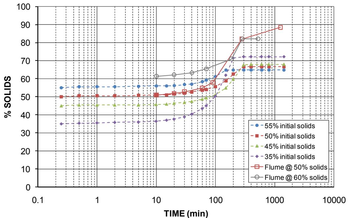
**Figure 37** Comparison of Swanbank fly ash average % solids on settling column, and flume testing under water and under a high head
