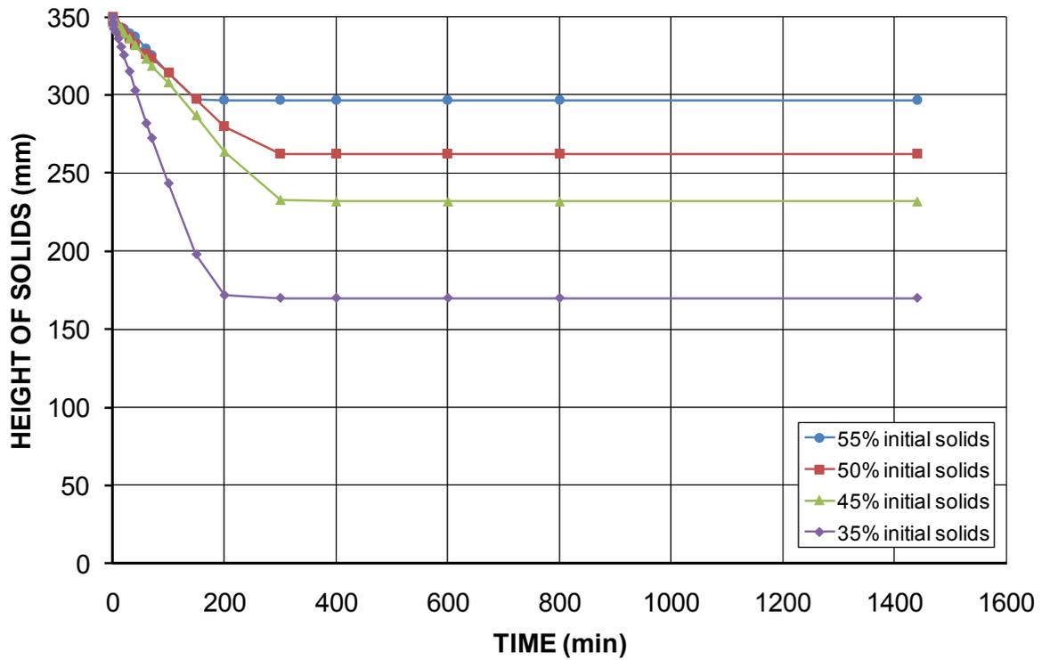
Figure 9 Settlement of Swanbank fly ash solids vs. Time for various initial % solids
