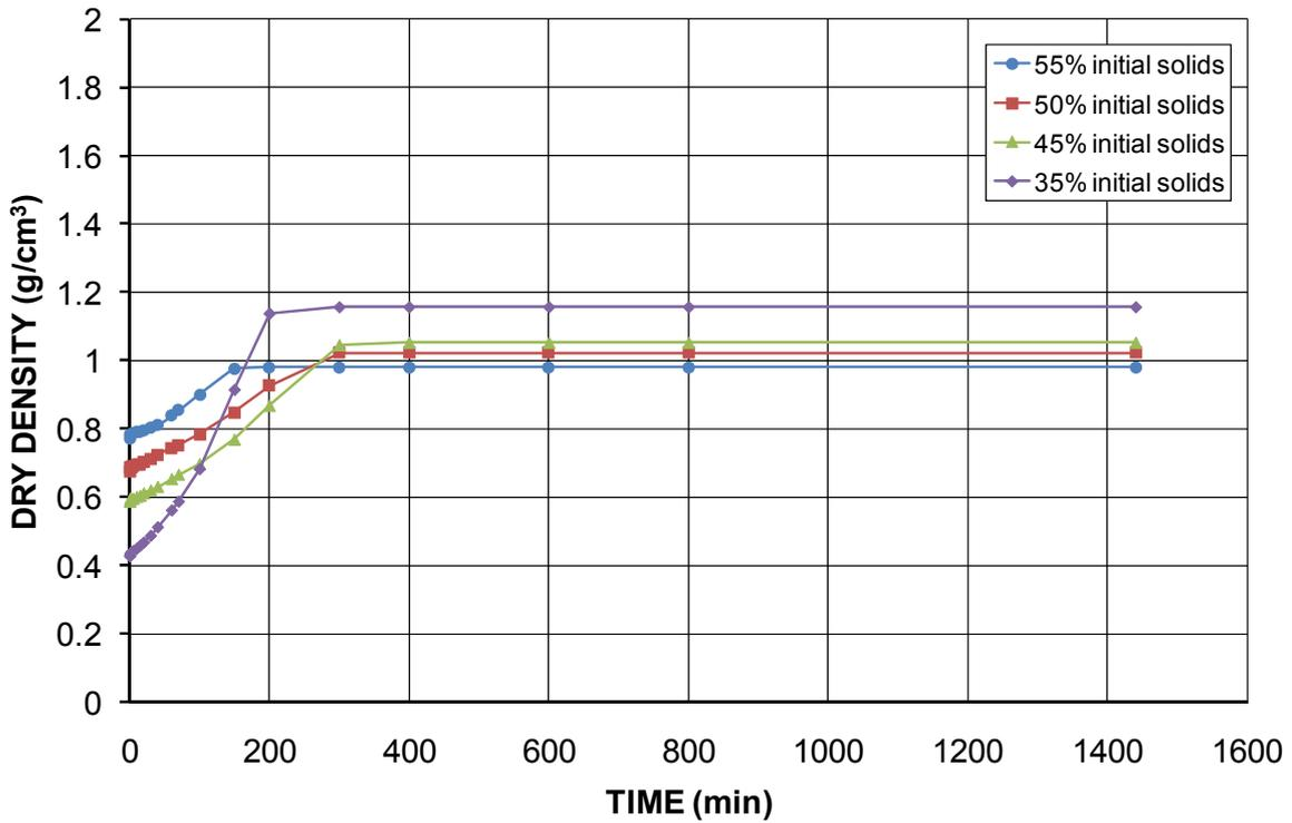
Figure 15 Average dry density of settling Swanbank fly ash solids vs. Time for various initial % solids
