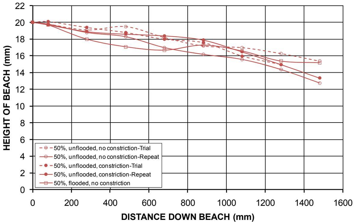
Figure 29 Summary of open-ended laboratory flume beach profiles for Swanbank fly ash
