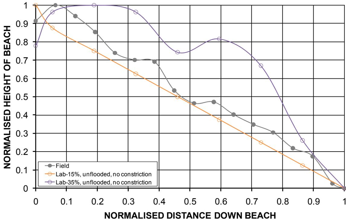
**Figure 41** Comparison of non-dimensional field and laboratory beach profiles for sub-aerial, unconstricted deposition of Swanbank fly ash
