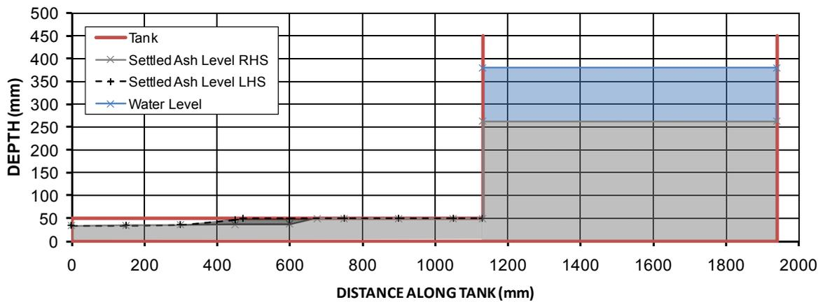
**Figure 36** Constricted backfilling, under water and a high head of Swanbank fly ash slurry, initially at 60% solids
