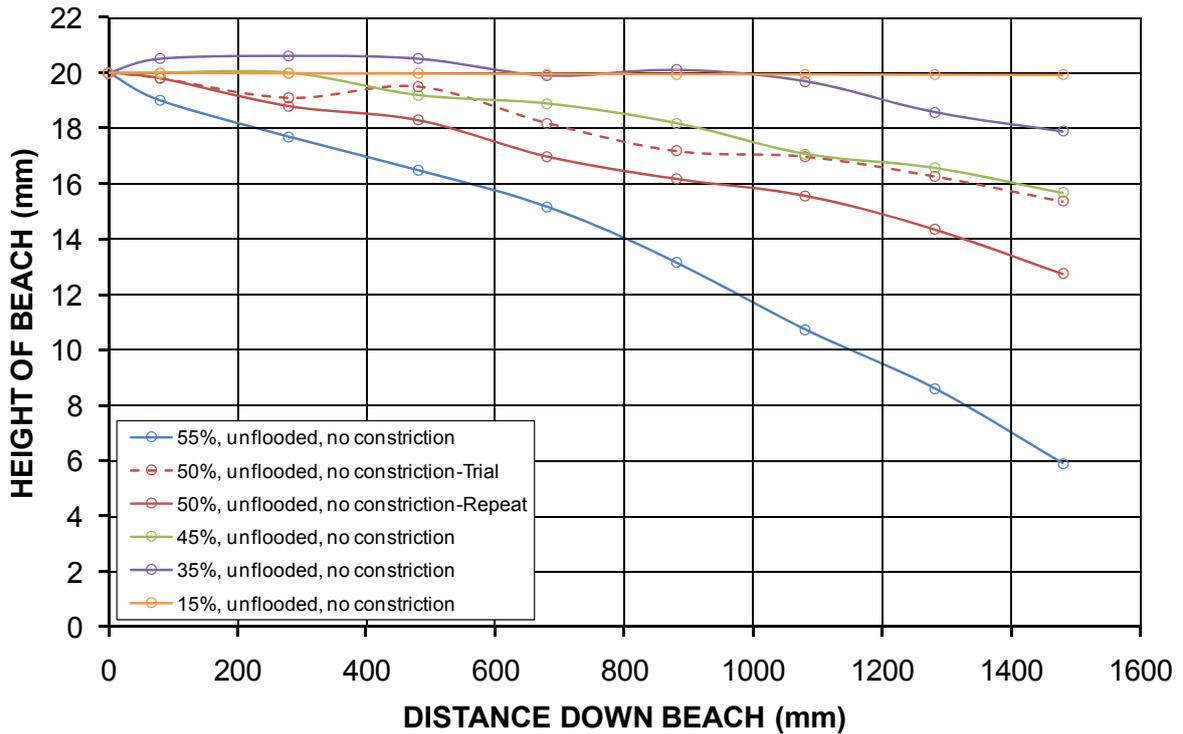
**Figure 31** Laboratory flume test beach profiles for unflooded, unconstricted deposition of Swanbank fly ash
