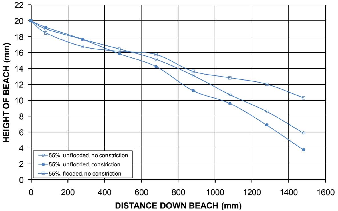
Figure 28 Summary of open-ended laboratory flume beach profiles for Swanbank fly ash
