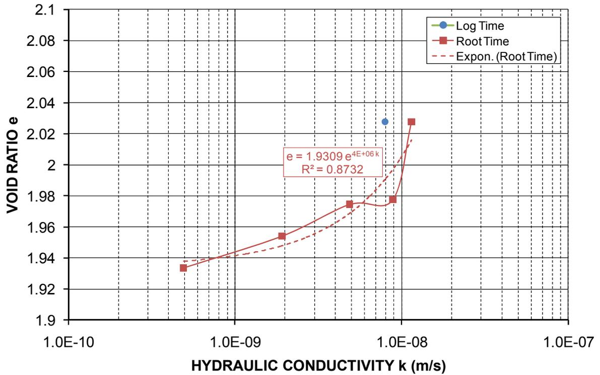
Figure 25 Void ratio vs. Hydraulic conductivity for Swanbank fly ash
