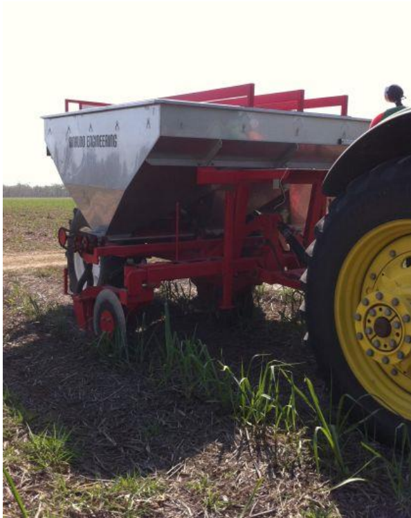
Fertiliser box – for accurate N placement
