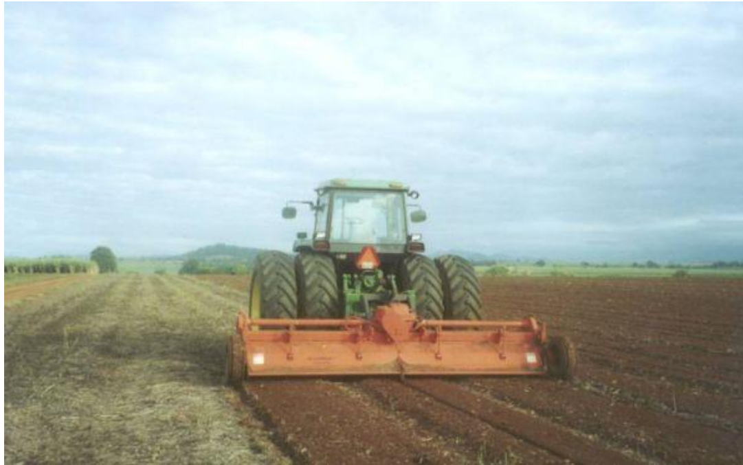
Zonal rotary hoe tilling three rows in one pass
