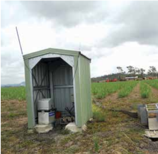
^ A Paddock to Reef Water Quality monitoring site with instrumentation to capture run-off
