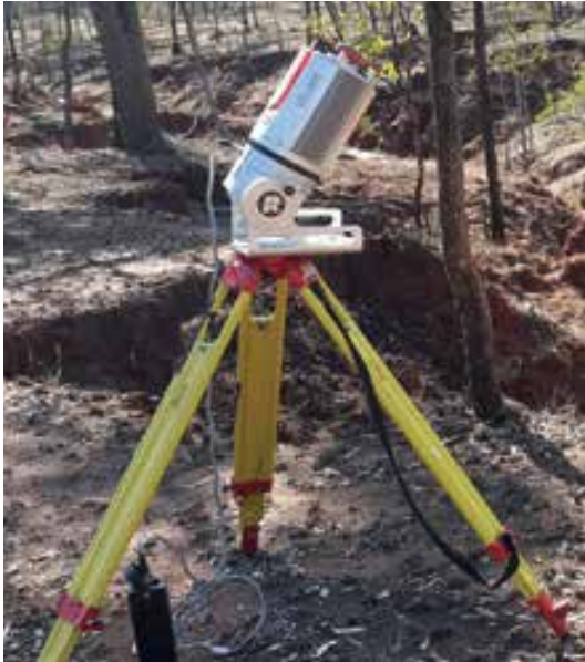
Scientists are developing approaches using this terrestrial laser scanner for highly detailed 3D monitoring of the changes in the gullies.
