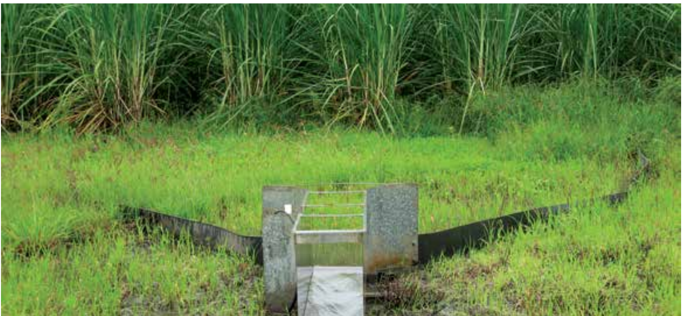
^ Measuring a run-off event through a flume set up at one of the Paddock to Reef Water Quality monitoring sites
