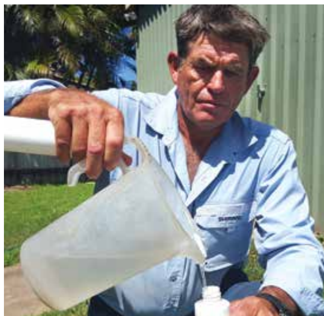
^ BBIFMAC staff member showing how to use a water quality monitoring kit to test for nitrates
