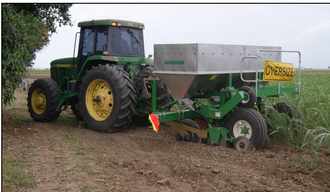
Figure 3: Fertiliser box supplied as part of the project being used to establish strips
