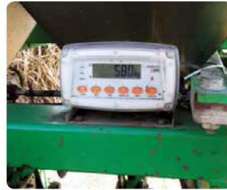
A fertiliser box has been specifically developed for this project. It includes load cells that allow Julian to monitor the amount of fertiliser which has been applied to each strip. This piece of machinery is a stool splitter and side dresser. It is not common place to use a commercial size piece of equipment to undertake research. This is yet another factor that makes this project unique.
