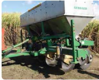
A fertiliser box has been specifically developed for this project. It includes load cells that allow Julian to monitor the amount of fertiliser which has been applied to each strip. This piece of machinery is a stool splitter and side dresser. It is not common place to use a commercial size piece of equipment to undertake research. This is yet another factor that makes this project unique.
