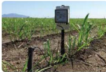
To gain a better understanding of irrigation management practices employed by farmers, soil moisture monitoring devices have been placed in all existing trial sites. These devices monitor soil moisture at various depths throughout the soil profile. The probes take regular readings, which are then downloaded and analysed. This information is invaluable in gaining a better understanding of the irrigation management practices employed by farmers involved in the trials and the impact this may have on final yields at each farm.
