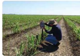
To gain a better understanding of irrigation management practices employed by farmers, soil moisture monitoring devices have been placed in all existing trial sites. These devices monitor soil moisture at various depths throughout the soil profile. The probes take regular readings, which are then downloaded and analysed. This information is invaluable in gaining a better understanding of the irrigation management practices employed by farmers involved in the trials and the impact this may have on final yields at each farm.
