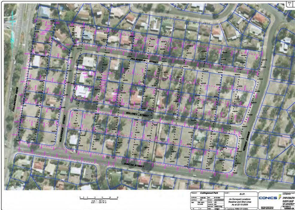
Figure 2-7. The actual 3D seismic survey layouts of receiver and shot lines. The magenta dots are shot locations while the black dots crosses are the receiver/geophone locations.
