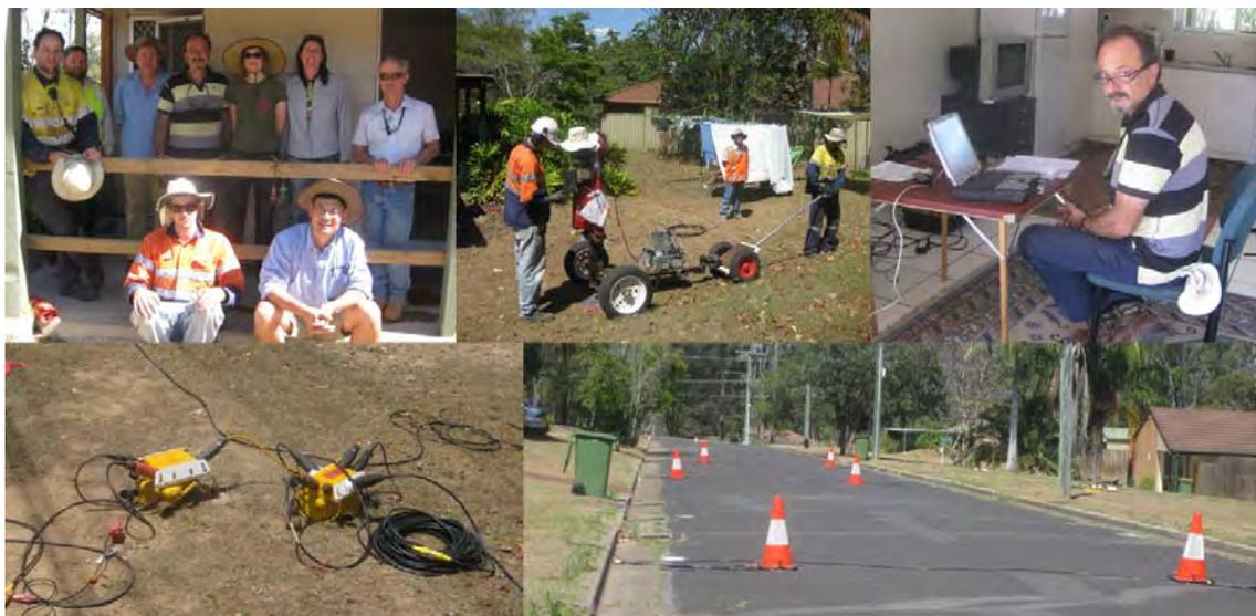
Figure 2-6. Seismic surveying in action at Collingwood Park. Top left: the seismic team; Top middle: Shooting in the backyard with accelerated weight drop device Digipulse 120 AE; Top right: Seismic recording computer; Bottom Left: Line cables, Line Tap Unit, Acquisition Unit and Batteries; Bottom right: Seismic receiver line running across the road and geophones (next to the traffic cones) planted on the road.
