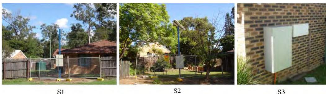
Figure 4-2. Microseismic stations S1, S2 and S3. The data acquisition system and battery are within the enclosure. The battery is charged using a solar panel installed on the top of the post.
