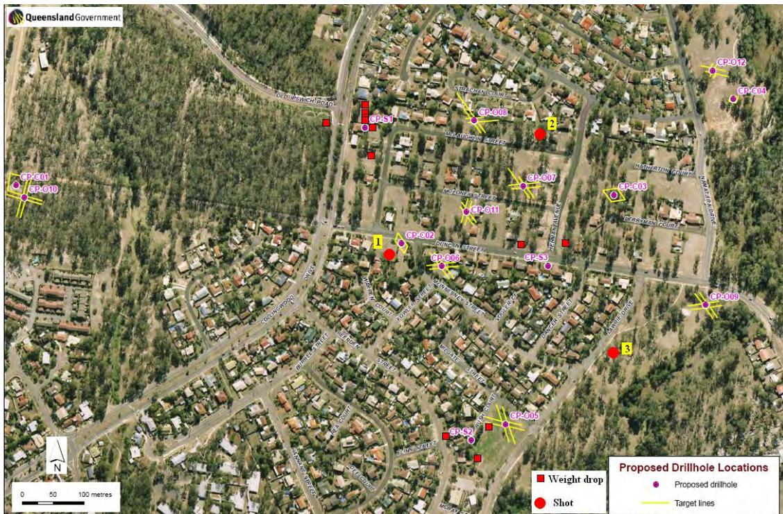
Figure 4-1. Locations of three geophone boreholes CP-S1, CP-S2 and CP-S3, weight drop points (red square) and suggested shot holes (large red dots).
