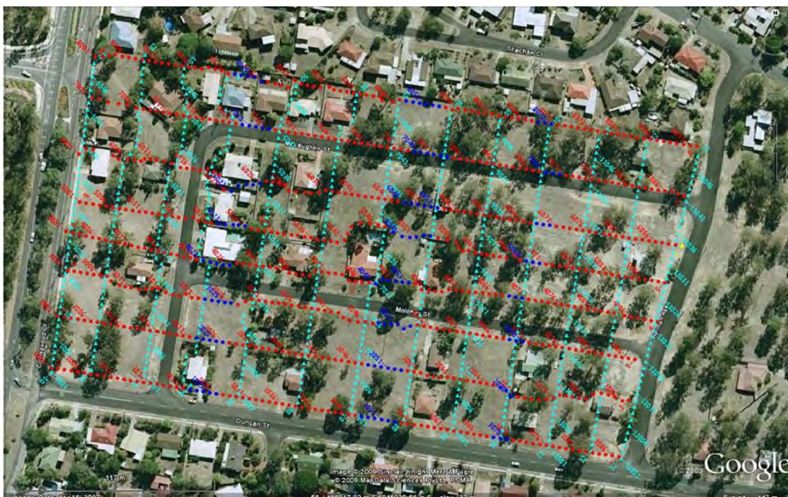
Figure 2-3. Basic 3D seismic survey layout of receiver and shot lines. The red/blue dots are the designed shot locations while the light-blue triangles are the receiver/geophone locations. The blue shot points are designed for repeating shots.
