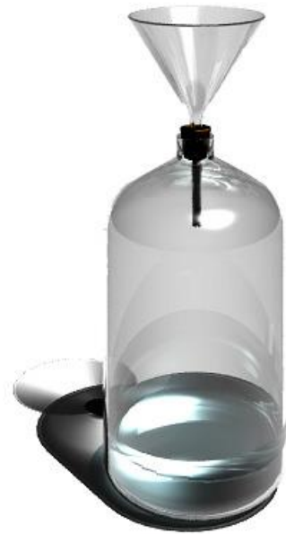
Figure 4: Dust gauge bottle and funnel.
