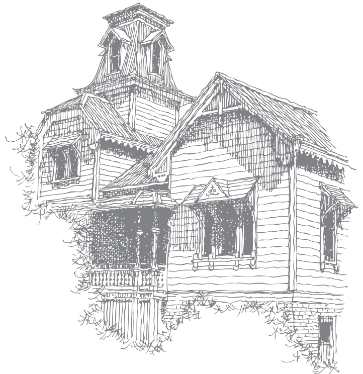
The roof of the Victorian house often drew attention to itself with varied forms, steep pitches, gables and decoration
