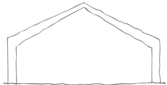
Typical portal frame—material could be timber (laminated or ply), steel or concrete
