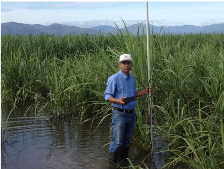
Figure 51: Measuring flow in sugarcane farms using a hand held flow tracker.
