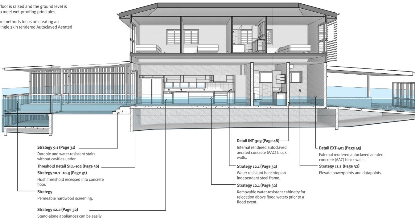
Masonry | Rendered AAC block
