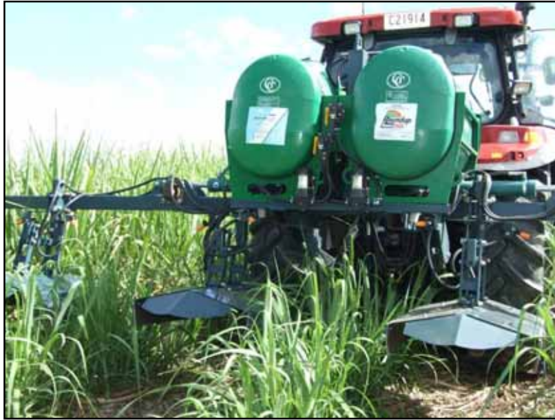
Figure 2-8. The control of weeds using shielded sprayers is being encouraged as an improved management practice in the sugar industry. This approach targets weeds early, reduces the total amount of herbicide applied to the paddock, uses products less susceptible to runoff (e.g. glyphosate), and reduces the need for residual herbicide control. Photo: B. Masters
