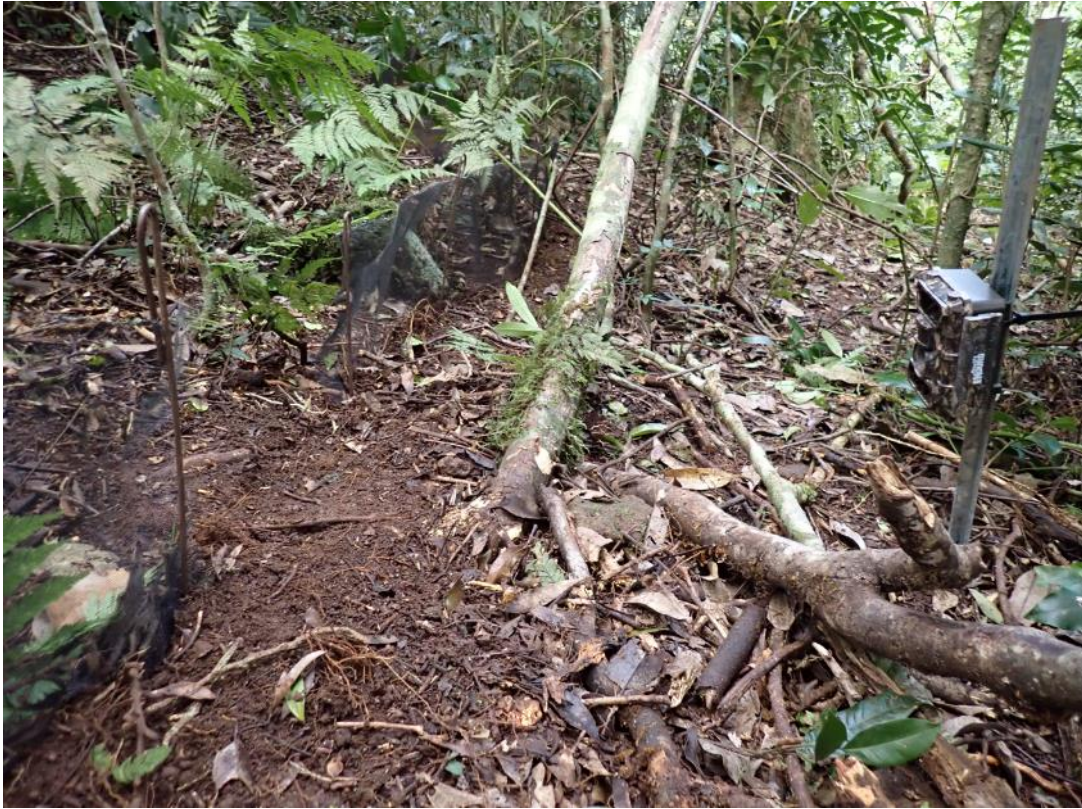
Figure 42: Close-focus black-flash camera trap on drift-fence. Note the break in the fly-wire drift fence and cleared leaf litter in the camera's focal zone. (Photo: M. Venz)
