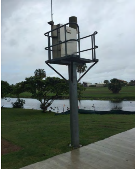
Figure 3.5 POLE MOUNTED STREAM WATER LEVEL AND RAIN GAUGE
