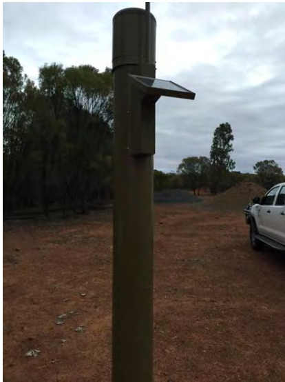
Figure 3.2 POLE MOUNTED PLUVIO CONNECTED TO ALERT NETWORK
