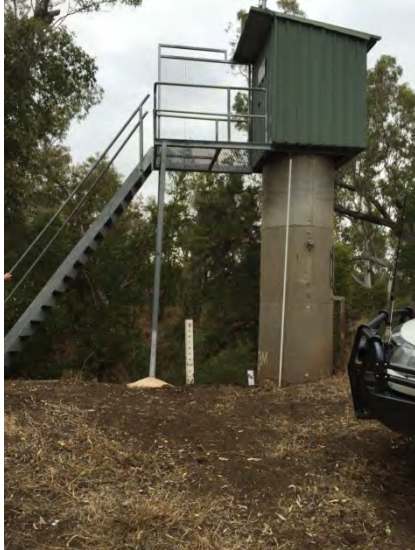
Figure 3.7 DNRM STATION FOR MEASURING STREAM WATER LEVEL AND RAIN, WITH STAFF GAUGE IN THE BACKGROUND
