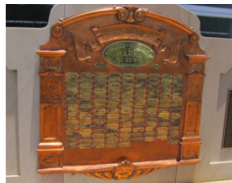
Locating a metal honour board outside can present special challenges when it comes to controlling corrosion. The brass name tags on this pressed copper honour board are tarnishing.
