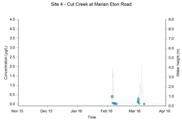
Figure 7-5 Hydrographic plot of water level and concentration ( \mu\text{gL}^{-1} ) of imidacloprid in Cut Creek.
