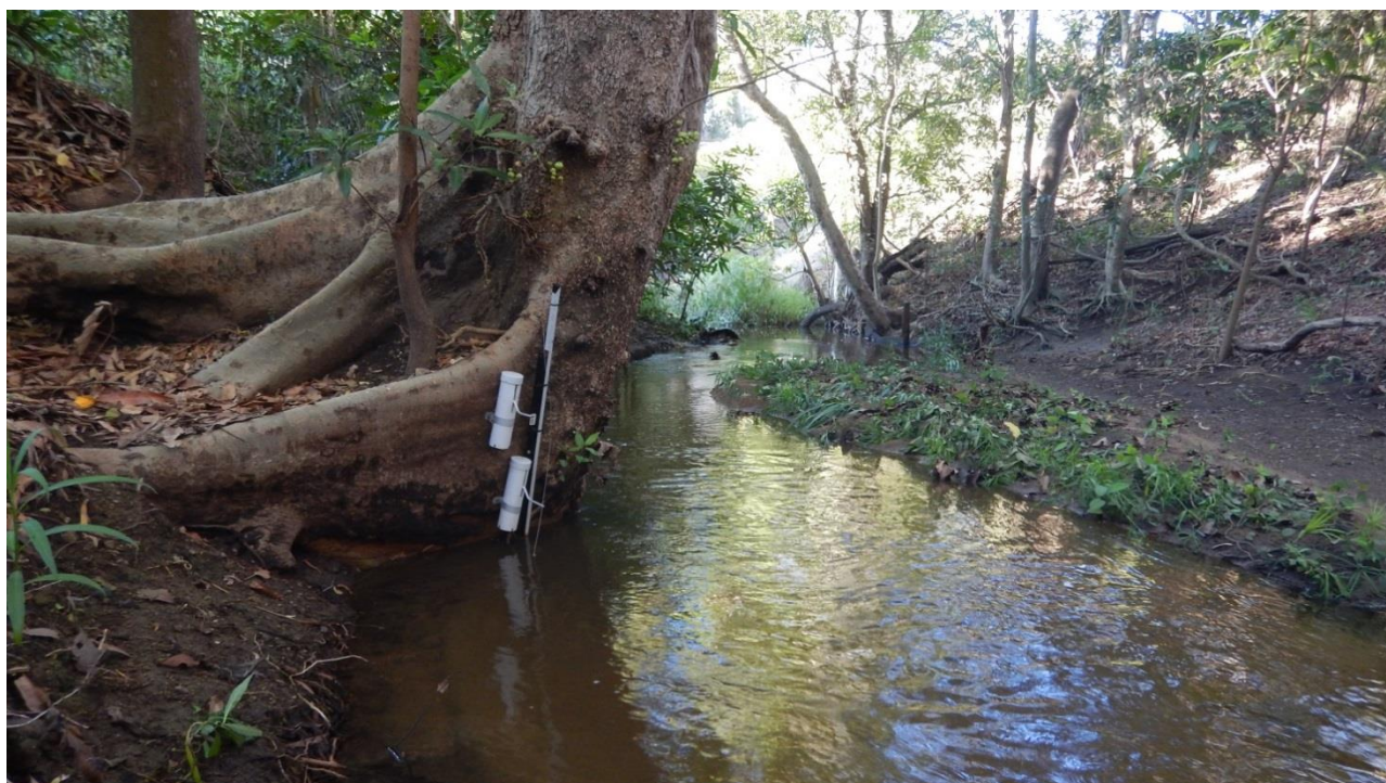
Figure 2-4 Water depth logger and rising stage samplers installed in Sandy Creek South Branch on the downstream side of a tree.
