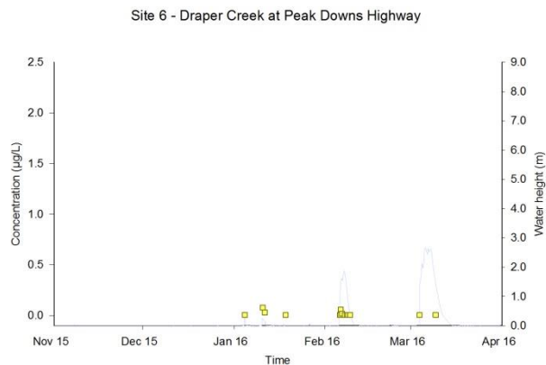
Figure 7-175 Hydrographic plot of water level and concentration ( \mu\text{gL}^{-1} ) of imazethapyr in Draper Creek at Peak Downs Highway.
