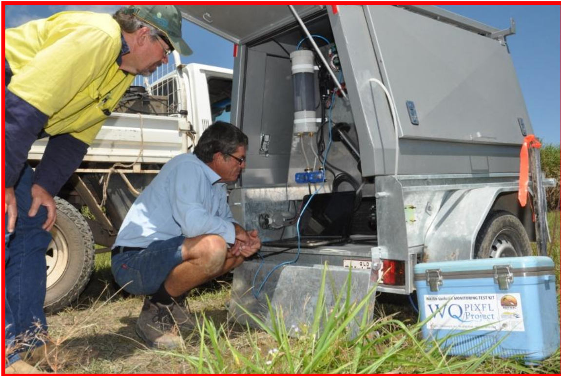
Figure 13. Project staff undertaking routine maintenance on the real time water quality monitoring trailer on site (photo credit: MSF Sugar).
