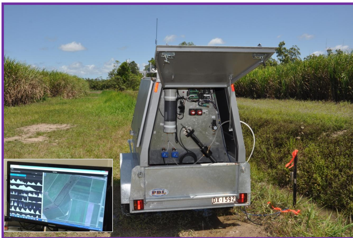
Figure 3. Real Time Water Quality Monitoring Trailer and Agtrix on-line database output (inset).
