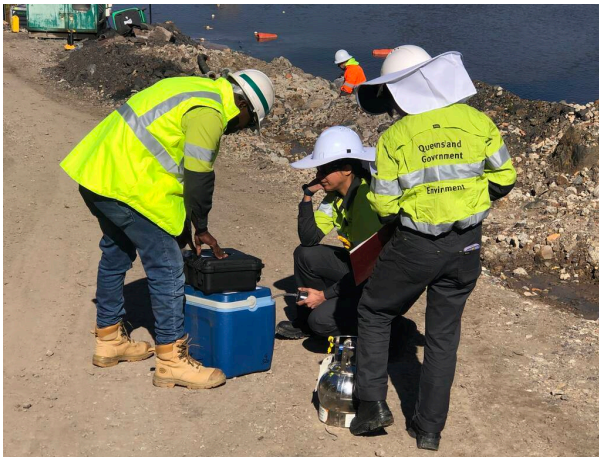
DES staff on-site at Cleanaway New Chum taking air samples using the new technology and, for comparison of results, the current canister technology (the silver spherical device on the ground).
