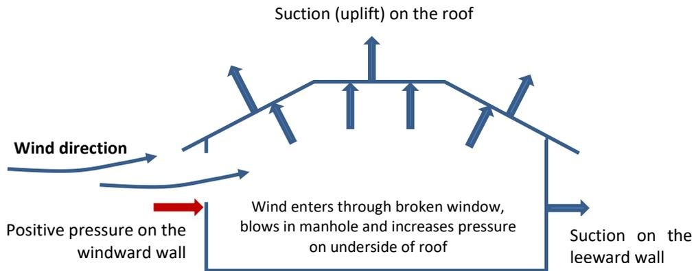
Figure 4 – Typical internal pressures on a building with an opening on a windward wall
