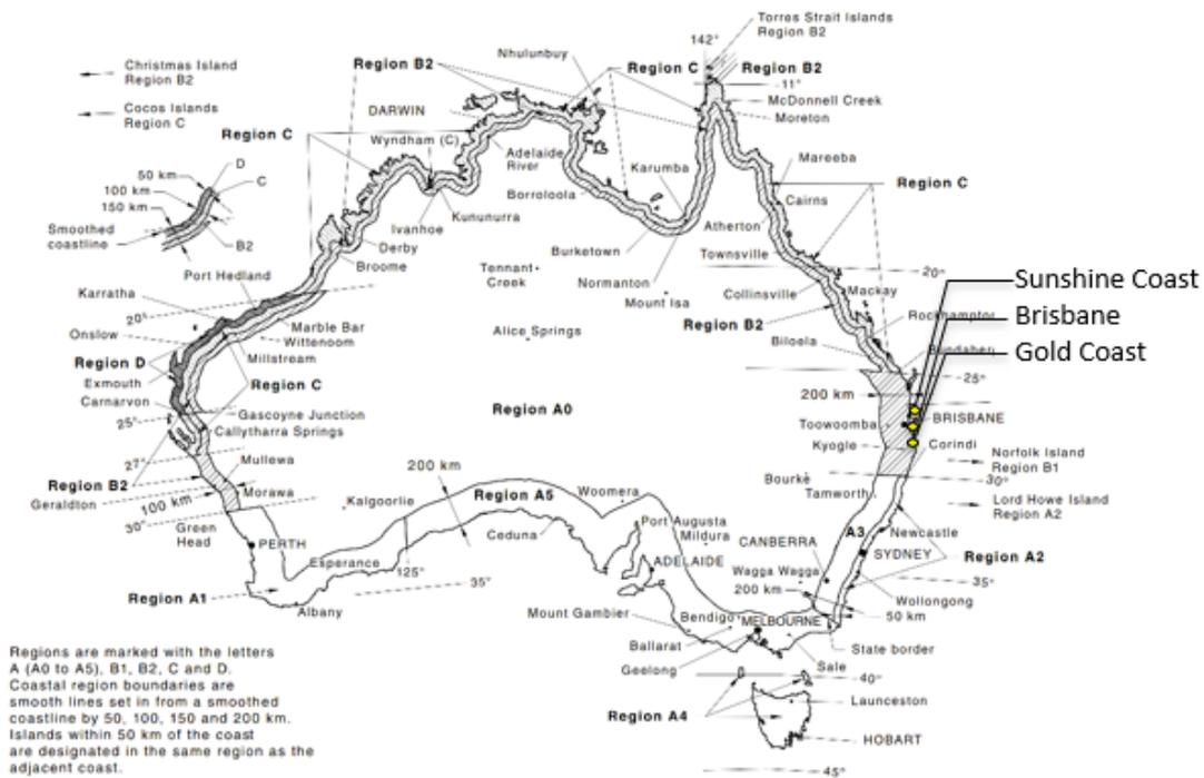
Figure 2 – Wind regions in Australia from Fig 3.1(A) in AS/NZS 1170.2:2021
