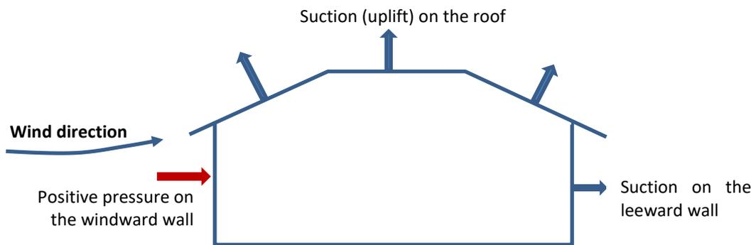
Figure 3 – Typical external pressures on a sealed building
